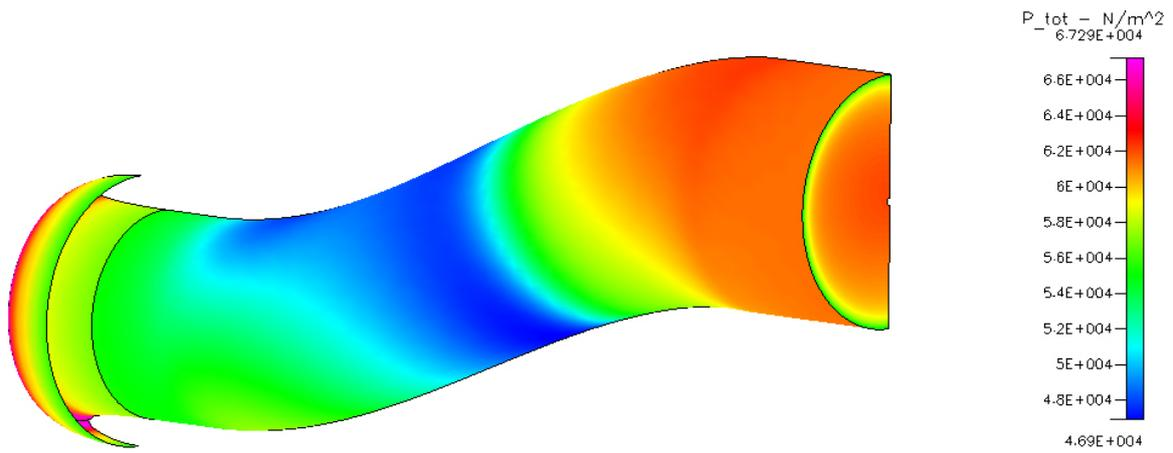
Fig.11.Total pressure contours on the optimal intake surface
