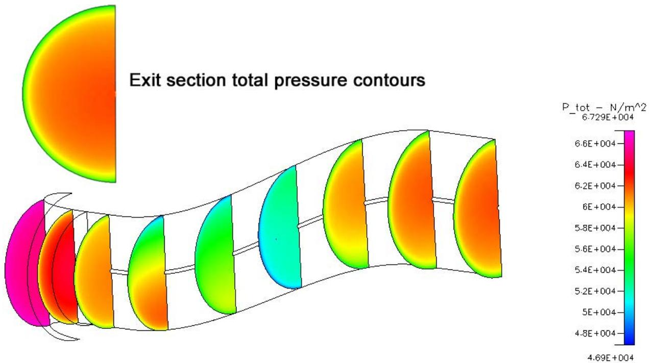
Fig.10.Total pressure sections contours for the optimal intake
