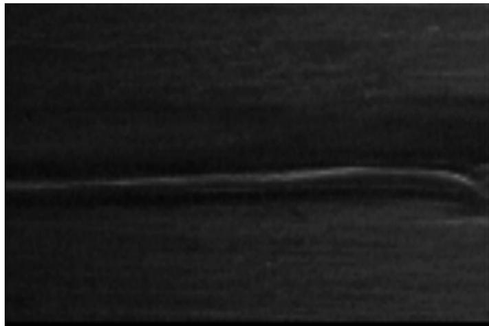
Fig.9. Optical Microscopic View of Fibre buckling under compression
