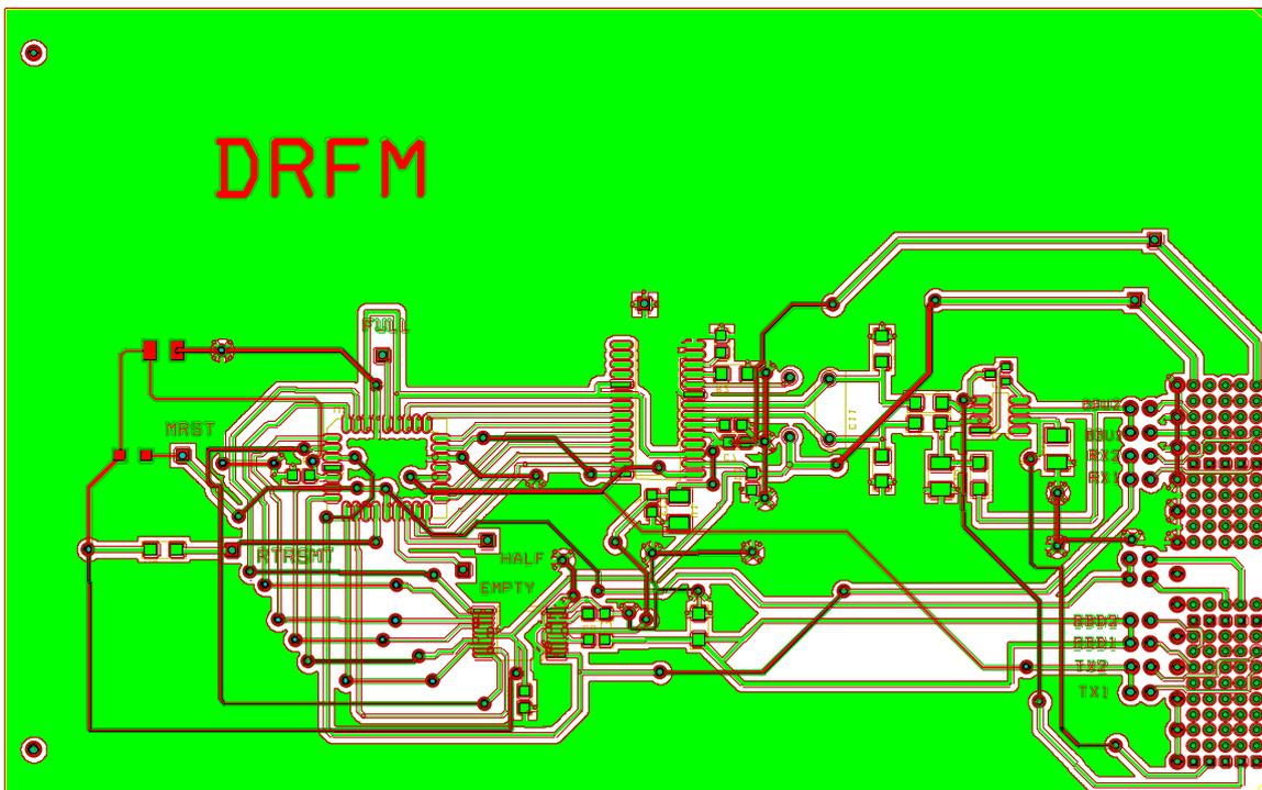
Fig. 9. A preliminary layout of the DRFM board
