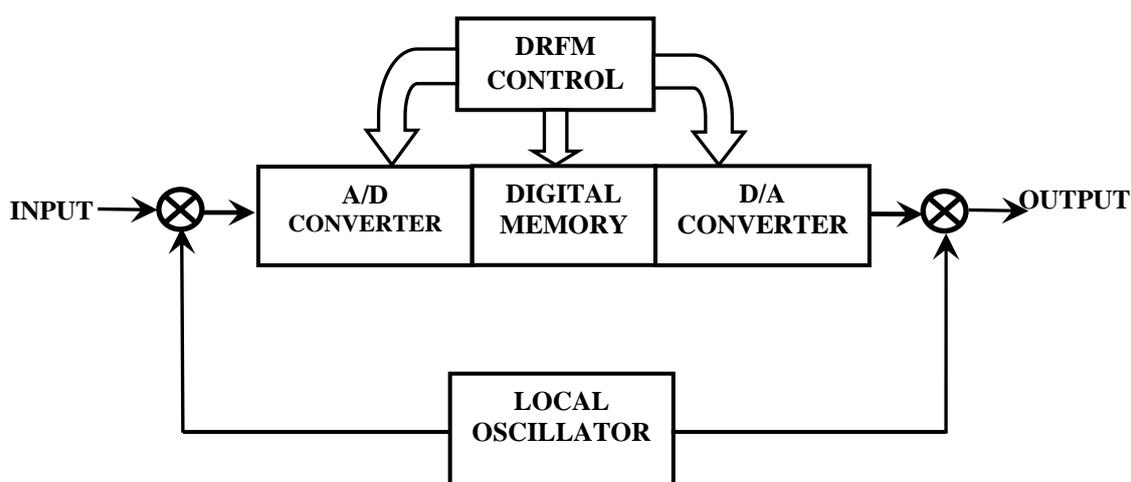
**Fig.1. Functional diagram of a frequency translation type DRFM system**
