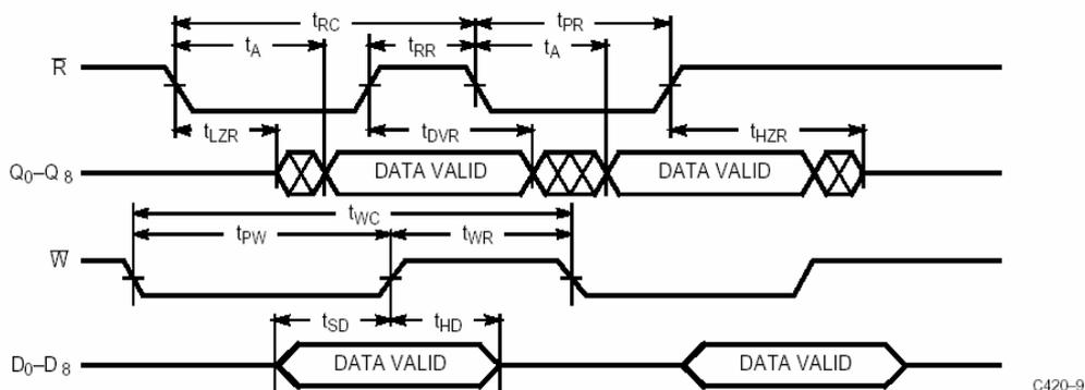
**Fig.5. Timing Diagram of the FIFO READ and WRITE**
