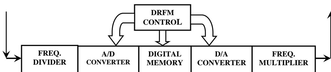
**Fig.2. Functional diagram of a frequency division/multiplication type DRFM**
