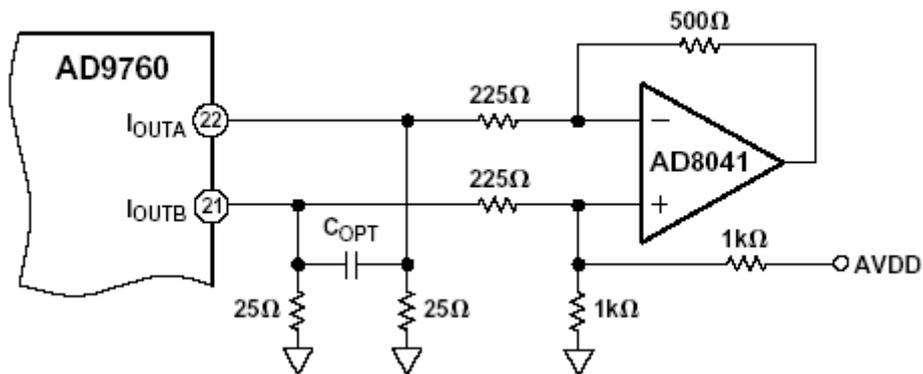
Fig.7. balanced-to-unbalanced conversion at the D/A output
