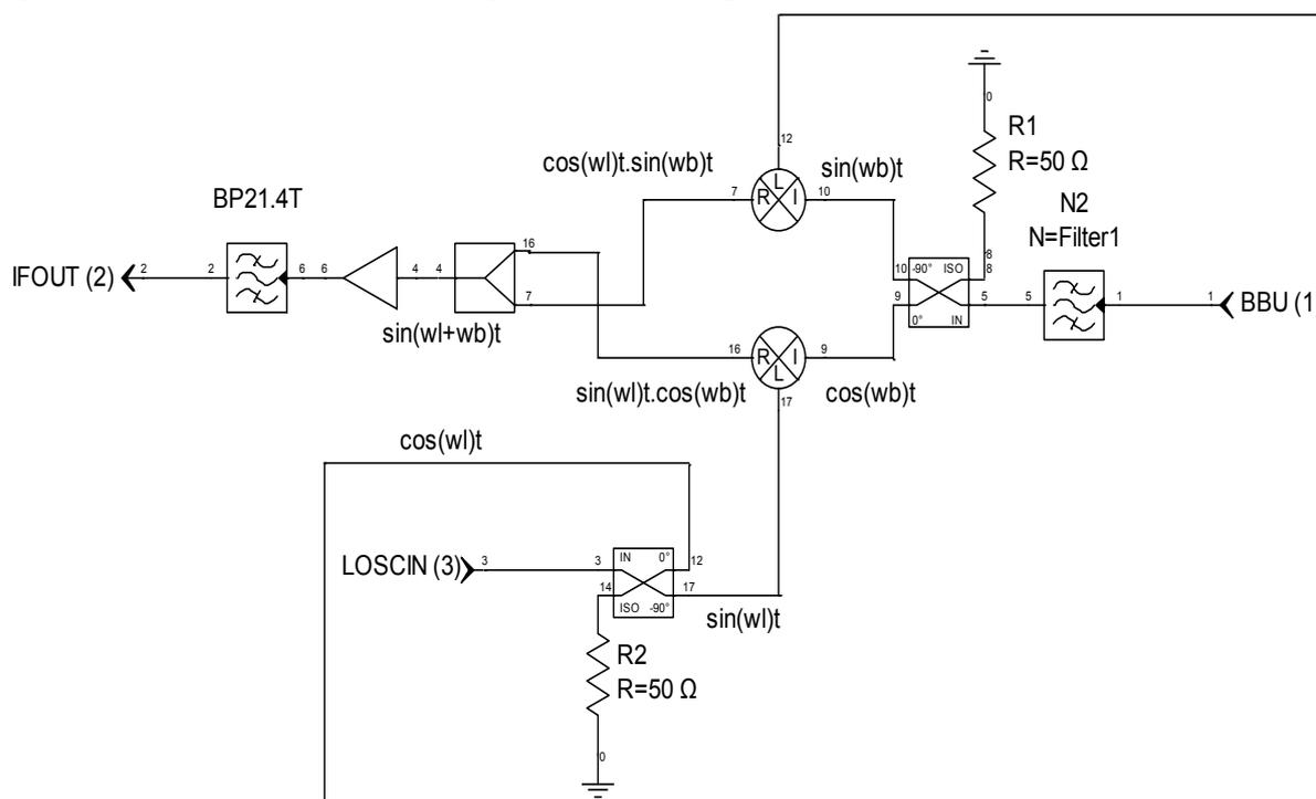
**Fig. 10. Functional diagram of the single-side-band up converter board**
