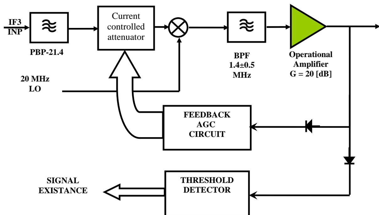
**Fig. 3. A Simplified Functional Diagram of the down conversion Board**
