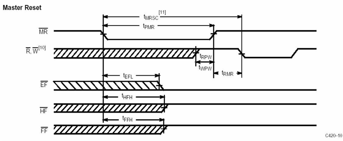
**Fig.4. Timing Diagram of the FIFO MASTER RESET**
