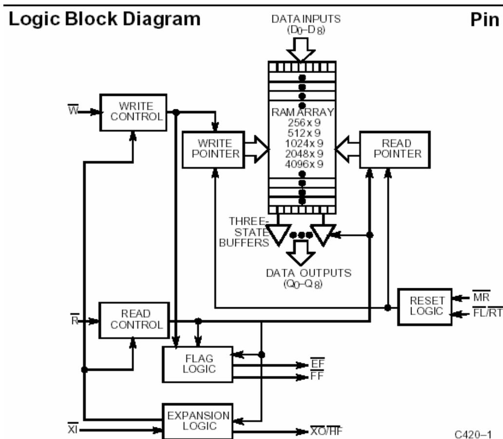
**Fig.6. Logical Diagram of the FIFO**
