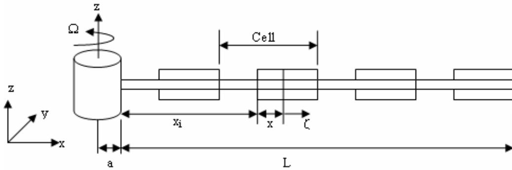
Figure 1: configuration of periodic rotating Timoshenko beam
