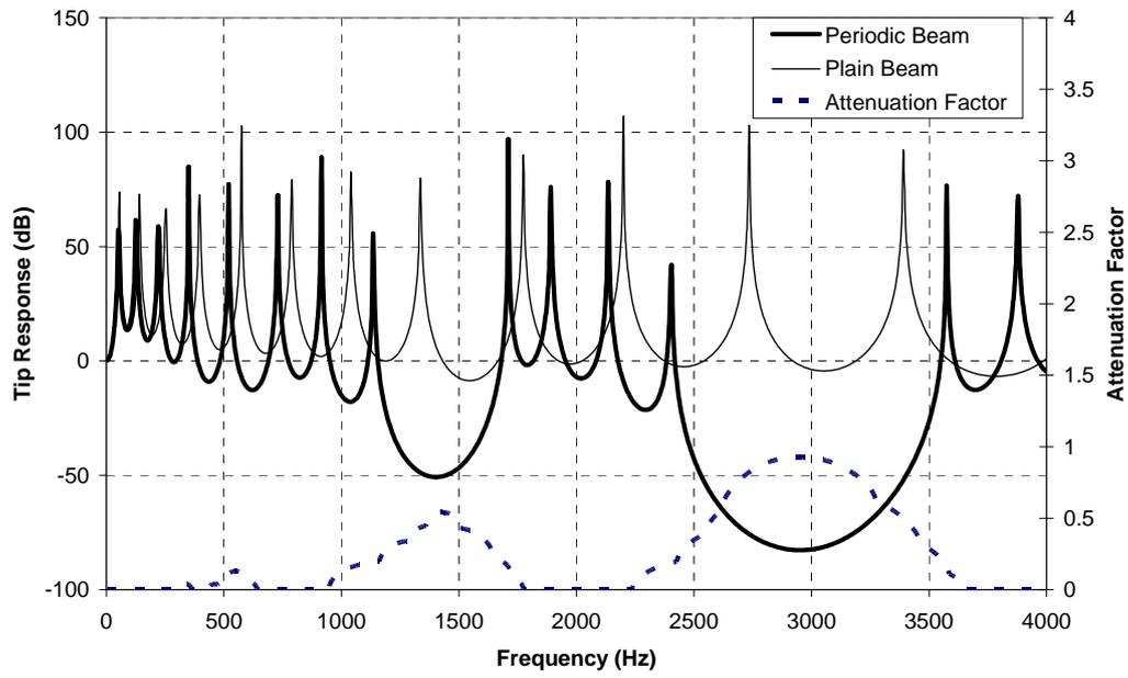
Figure 5: Frequency response of periodic rotating Timoshenko beam (50 rev/sec)
