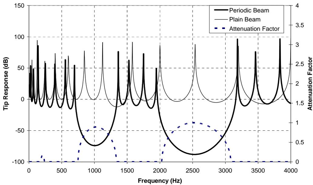
Figure 4: Frequency response of periodic rotating Timoshenko beam (5 rev/sec)
