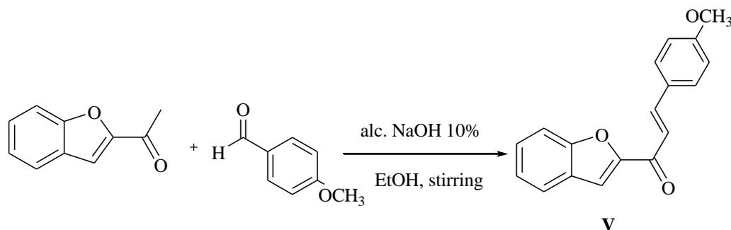
**Scheme (3):** Aldol condensation between 2-acetylbenzofuran and p-methoxybenzaldehyde to form chalcone **V**
