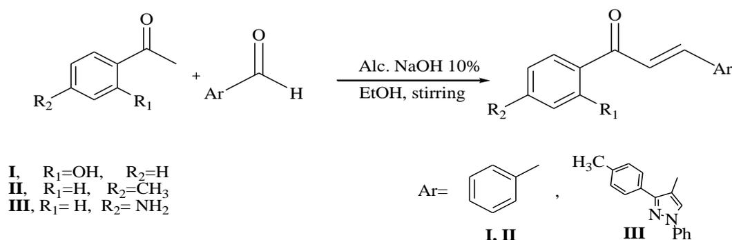
**Scheme (1):** Claisen condensation between aromatic aldehydes and aromatic ketones to form chalcones
