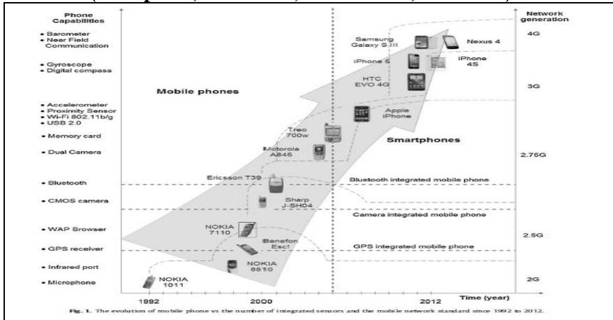
Fig. 1. The evolution of mobile phone vs the number of integrated sensors and the mobile network standard since 1992 to 2012.
