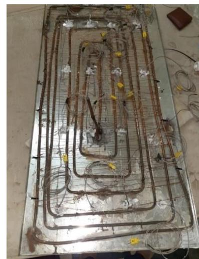
**Fig. 2. A rectangular helical shape of copper tube with fins.**
