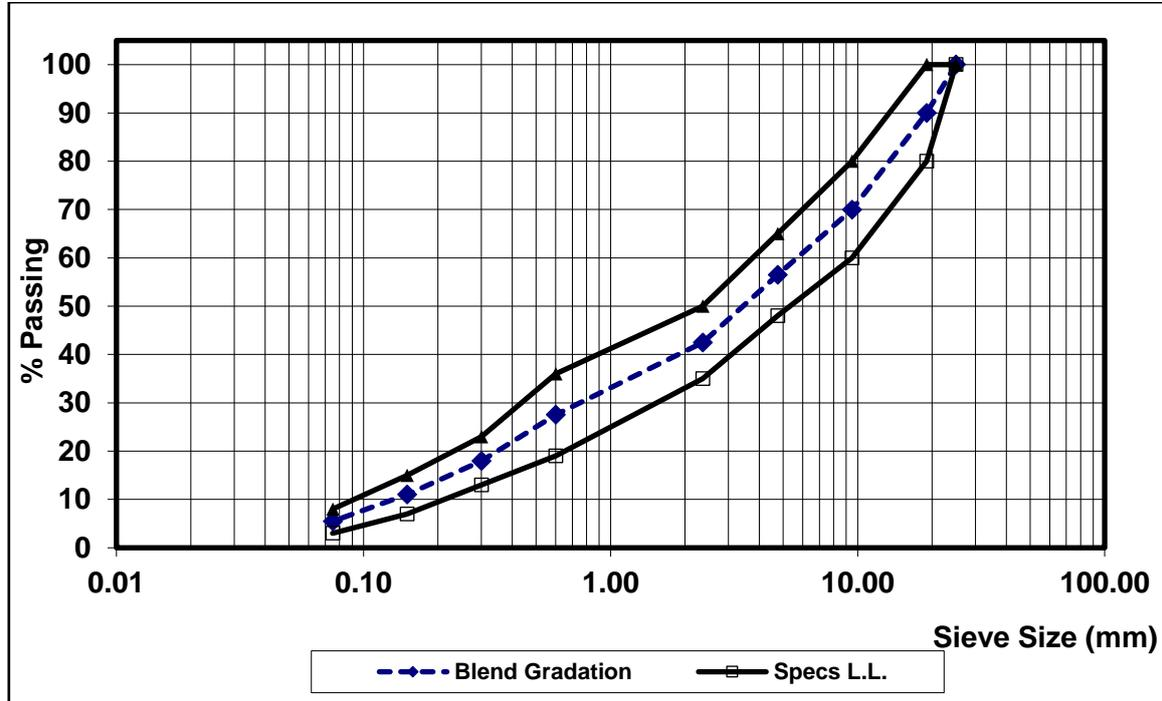
**Fig 1 :% Passing vs. Sieve Analysis for Blend and Specs Limits**
