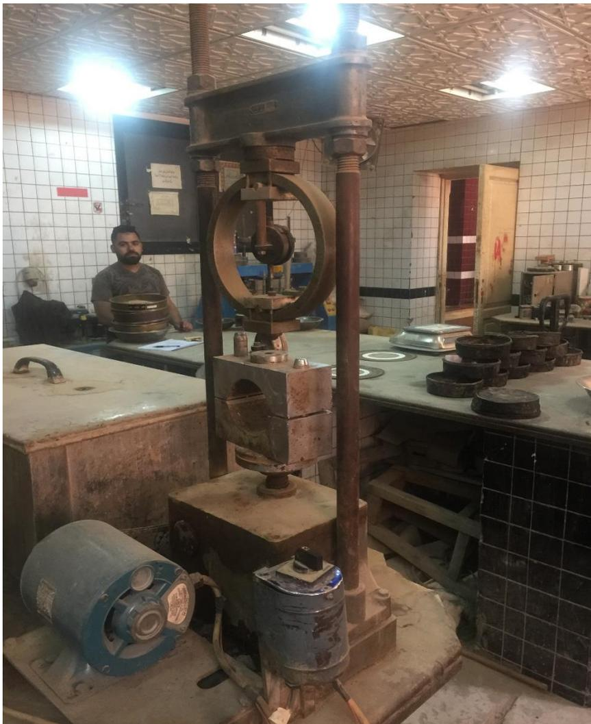
**Fig 2: Marshal stability- flow test**
