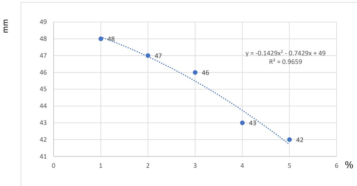
**Fig 6: The penetration test results for Crumb Rubber from recycled tires**
