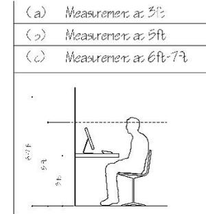
from the floor level of the worker's chair, to determine the average frequencies each worker is exposed to. Figure 10 Shows the different heights of each measurements (at 3 feet, 5 feet & 6/7 feet). Figure 11 shows the average of the 3 measurements at each desk's seat.
