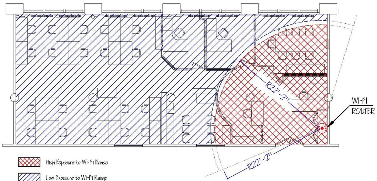
Figure 14: Recommended minimum distance of working desks from Wi-Fi routers.
