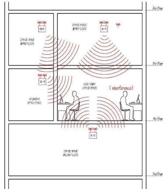
Figure 13: EM frequencies from other adjacent office spaces interfering and increasing exposure levels.
