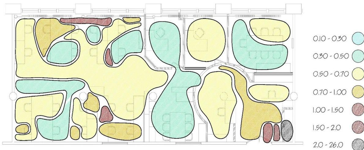
Figure 9: EM frequency measurements throughout the office space in v/m
