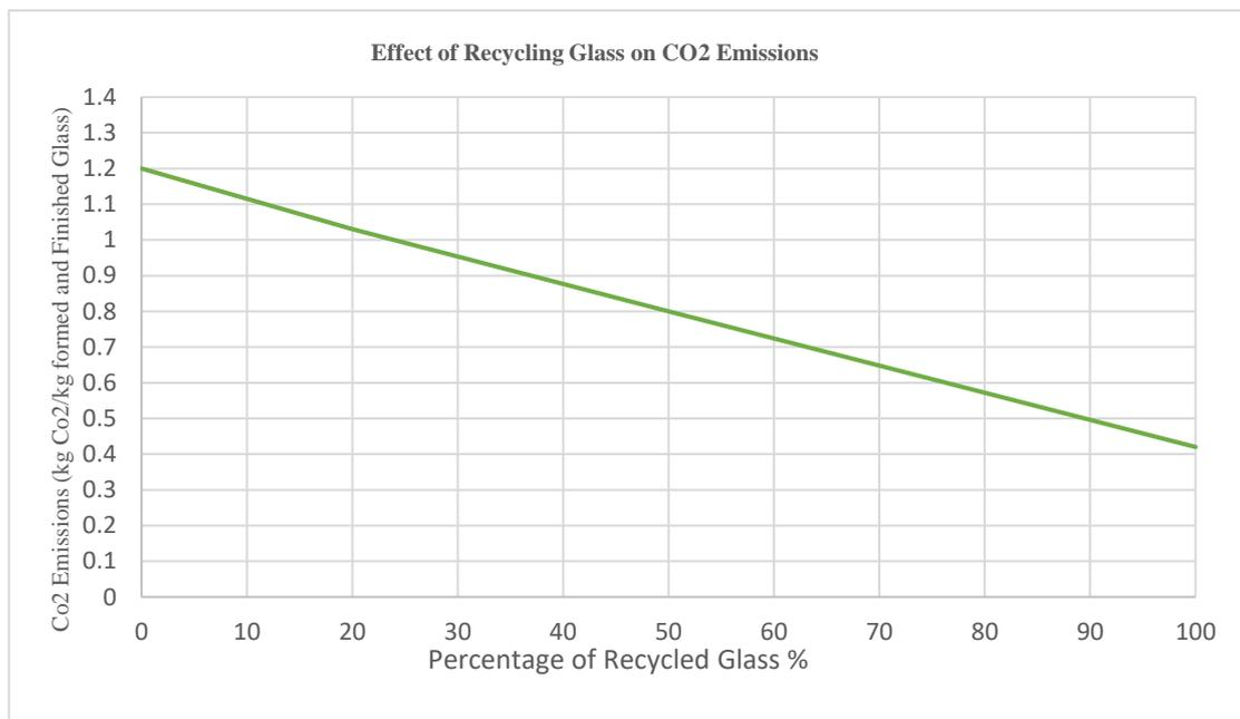
Figure 5. Effect of Recycling Glass on CO<sub>2</sub> Emissions [43].
