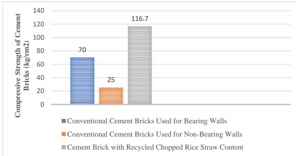
Figure 2. Compressive Strength of Cement Bricks (Comparison Between Cement Bricks for Load Bearing Walls, Non-Bearing Walls and Cement Bricks with Recycled Chopped Rice Straw Content).
