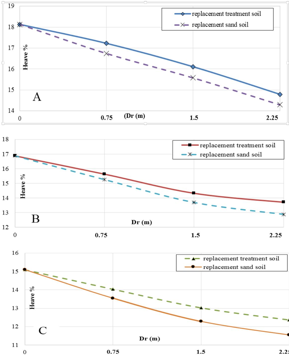
Fig. (3): Effect of replacement soil thickness on soil heave under
