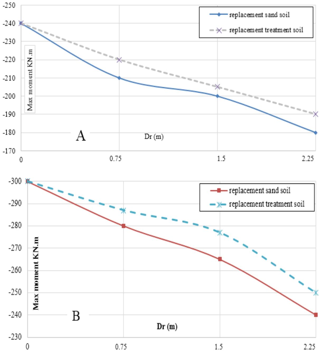
**Fig. (5):** Relationship between replacement soil thickness and maximum value of ground beam moment for
