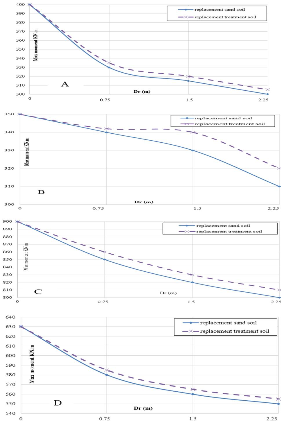
**Fig. (8):** Effect of replacement soil thickness on the maximum value of mat foundation moment along A- External column strips B- External field strips C- Internal column strip D- Internal field strips.
