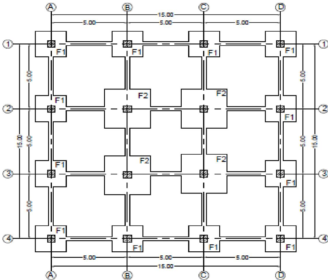
Fig. (2): plan view for the dimension of study structure and foundations models.
