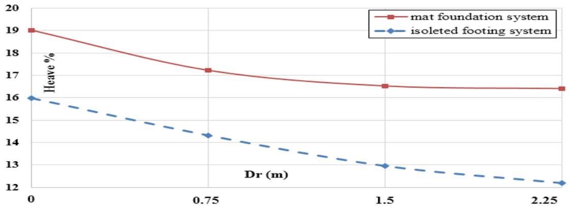
Fig. (9): The change in average value of soil heave percent due to change in thickness of the replacement sand soil for mat foundation system and isolated foundation system.
