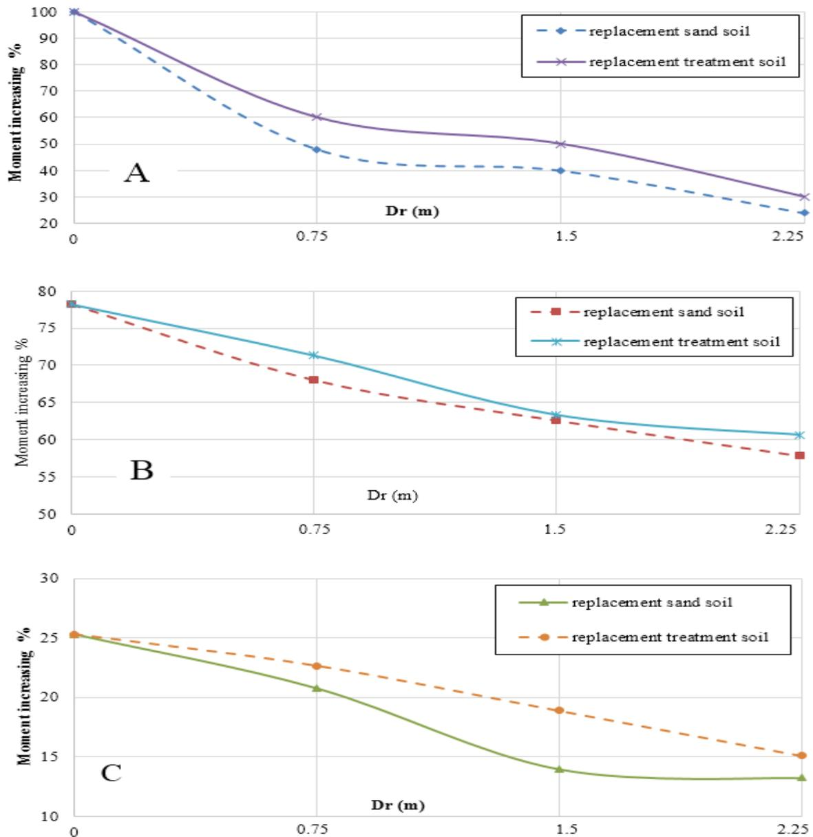
**Fig. (4):** Relationship between replacement soil thickness and increasing in footing moment for
