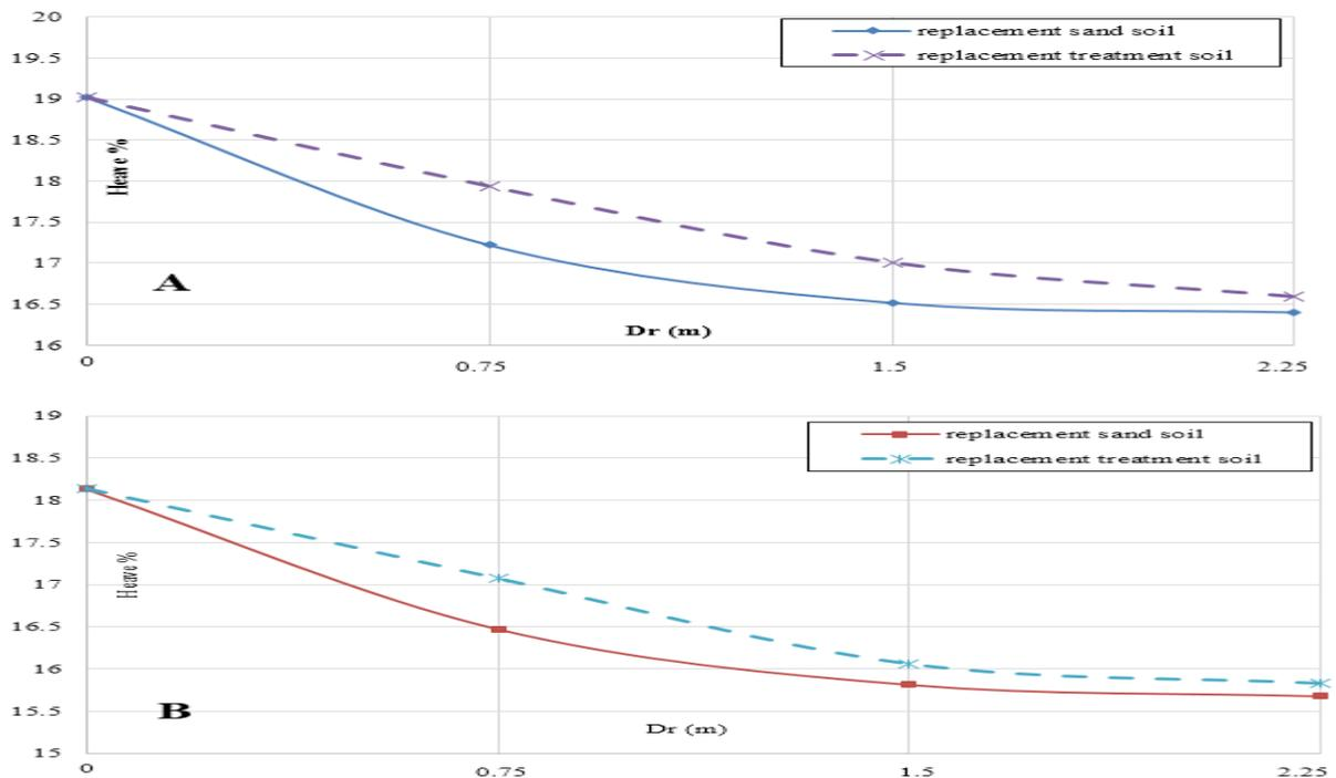
**Fig. (7):** The relationship between average values of soil heave percent for mat foundation and the replacement soil thickness along A- External field strips B-Internal field strips
