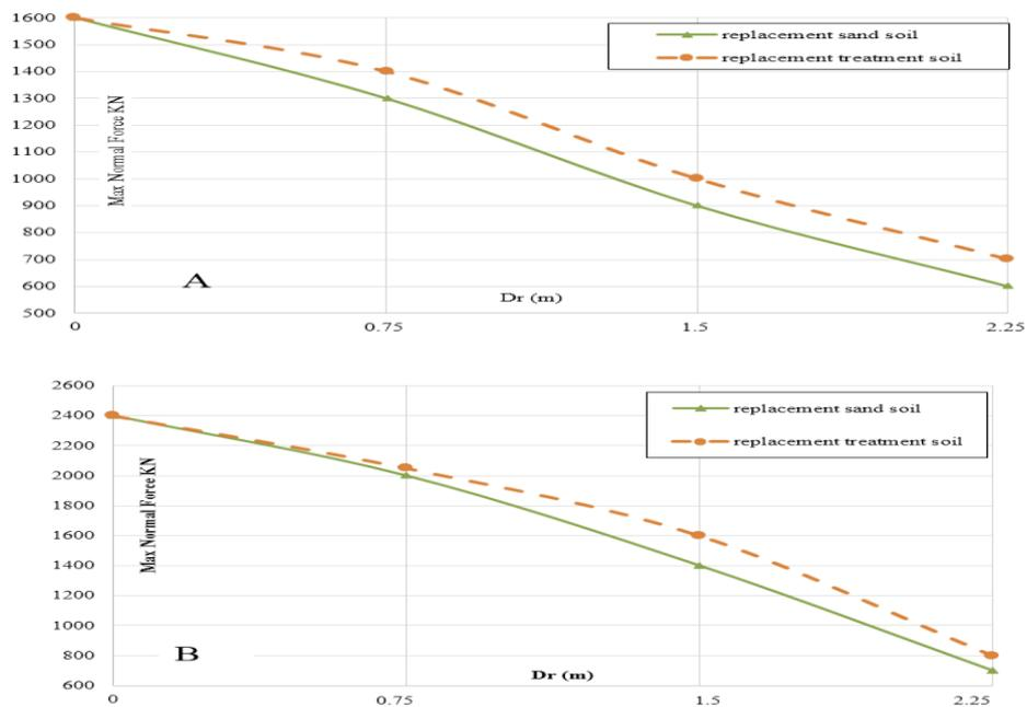
**Fig. (6):** Relationship between replacement soil thickness and maximum value of ground beam Normal force for A-External ground beam B-Internal ground beam
