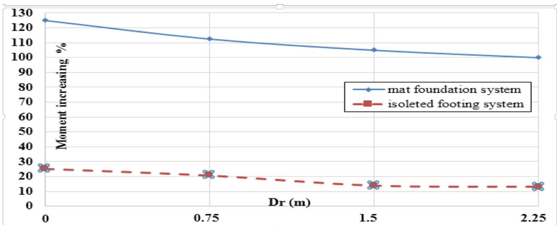
Fig. (10): The effect of change in replacement soil thickness on the maximum value of foundation moment for mat foundation system and isolated footing system.
