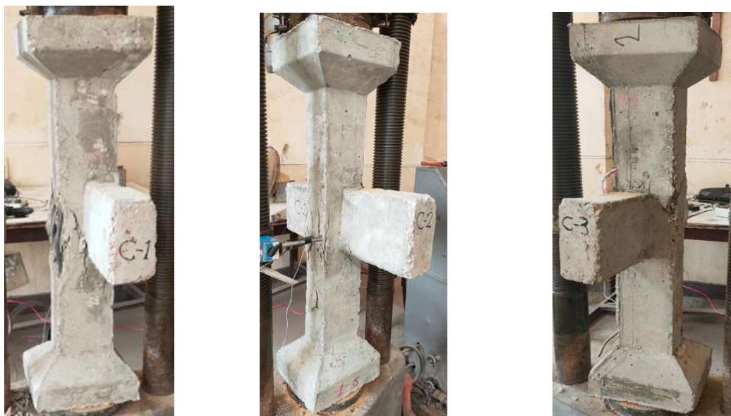
Figure 5 Cracks Pattern of Group 1 (C1-1&C1-2)
