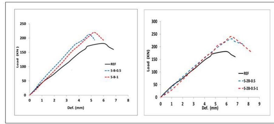
Fig.12. comparison of Load deflection based on the strengthening locations
