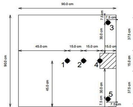
**Fig.7: Details and dimensions of line load.**
