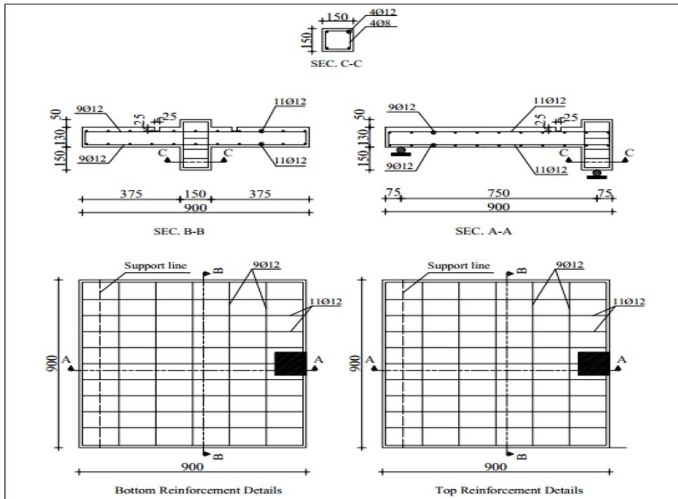
**Fig.2: Dimensions and reinforcement details for specimens**
