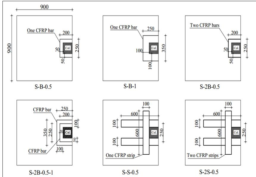
**Fig.1: Strengthening schemes (All dimensions in mm)**
