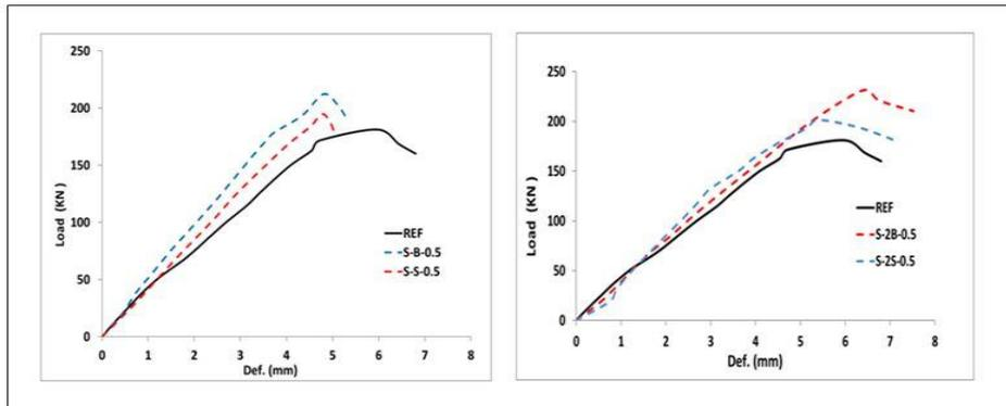
Fig.11: comparison of Load deflection based on the strengthening techniques
