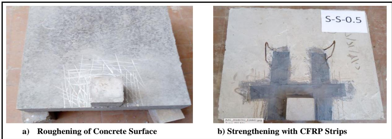
**Fig.5: Strengthening procedures using EB technique**
