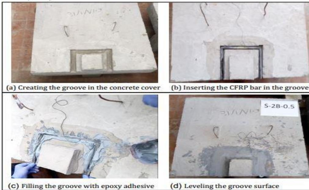
**Fig.4: Strengthening procedures using NSM technique**
