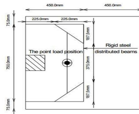
**Fig.9: LVDT locations at bottom side**
