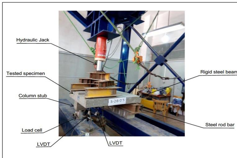
**Fig.10. Set-up of Test**
