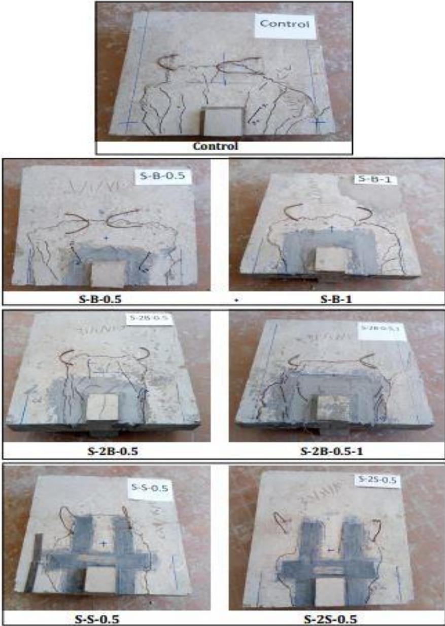
**Fig.14: The tested specimens crack patterns at failure load (bottom faces)**
