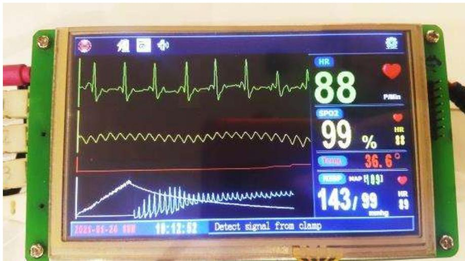
**Fig. 14:** The Data Displayed by Smart TFT
