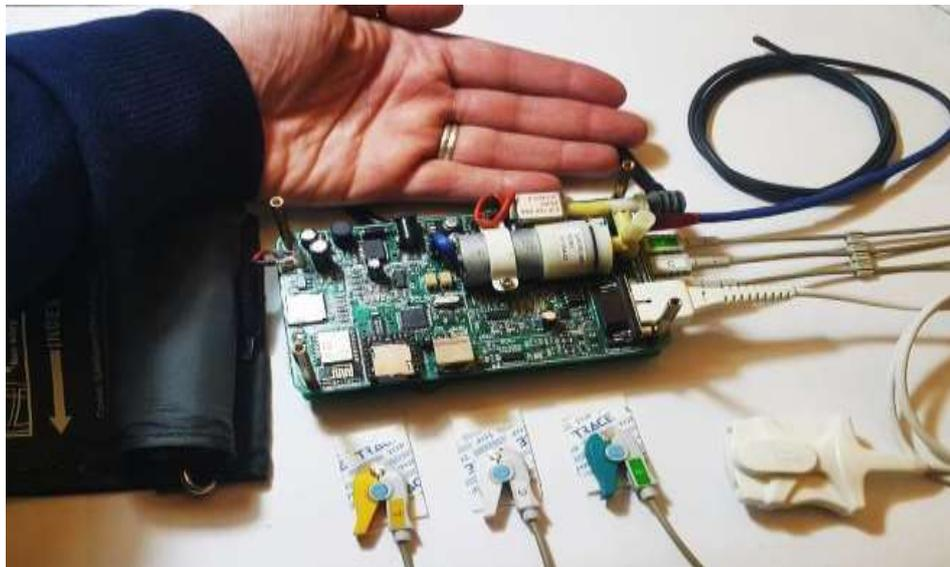
**Fig. 7:** Biomedical Handheld Embedded System Device
