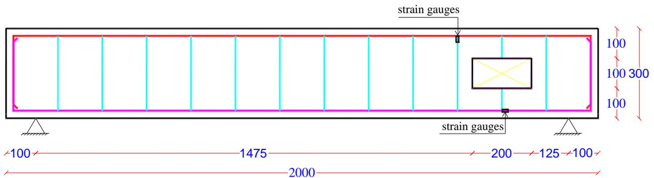
**Figure 6** The position of the Strain gauges.
