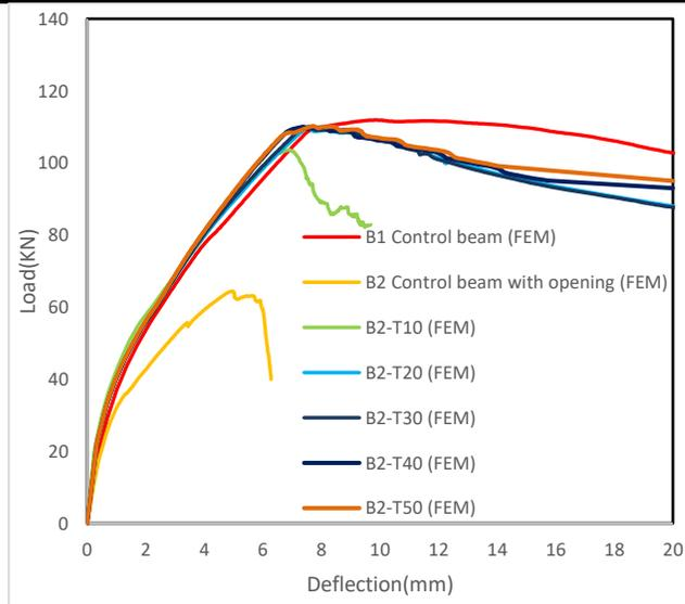
**Figure 20** the load-deflection relationship for the beam B2 with opening strengthening using different thickness from UHP-FRC plate.
