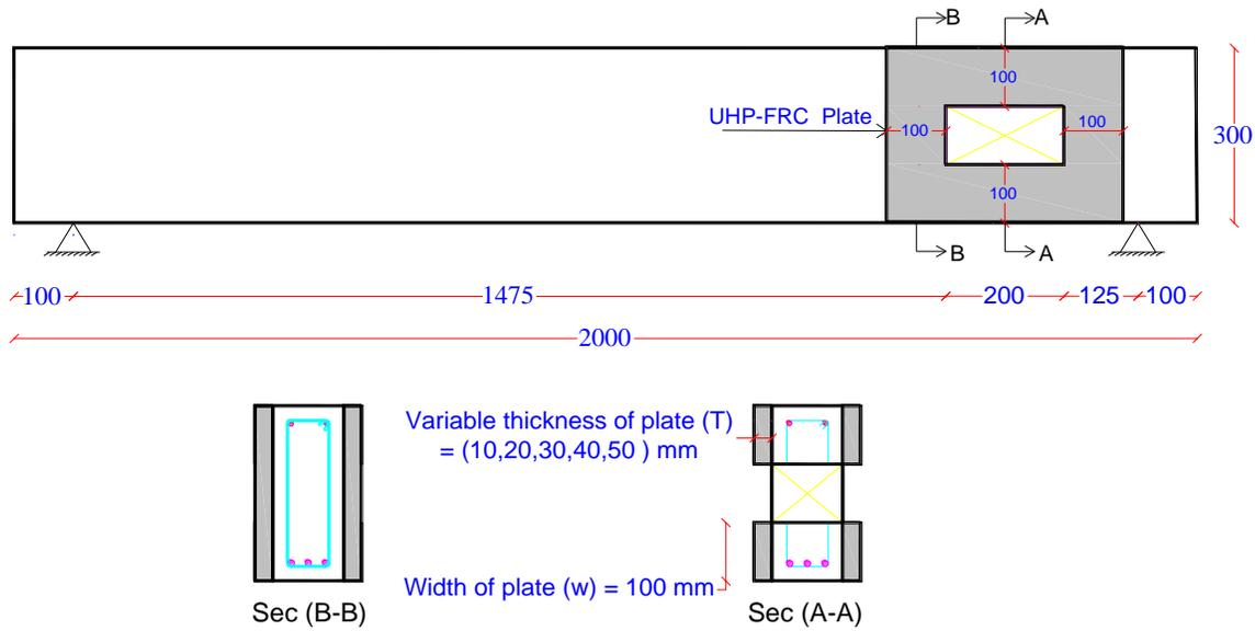
**Figure 4** Geometry and details of strengthened beams (B2) with opening for (Group 2) with different thickness UHP-FRC plate specimens.
