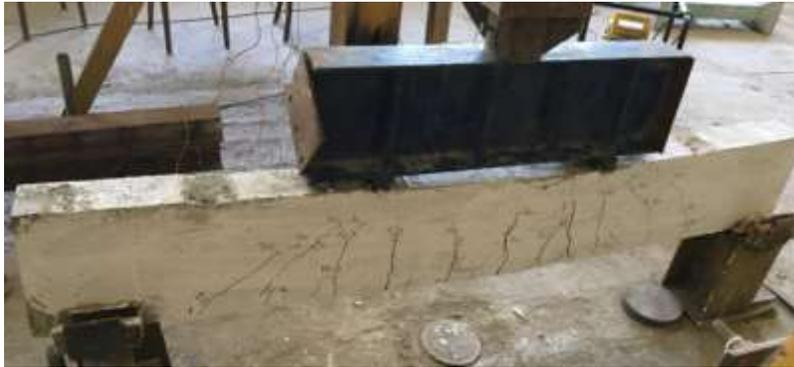
**Figure 7** Experimentall crack patterns of control beam (B1)
