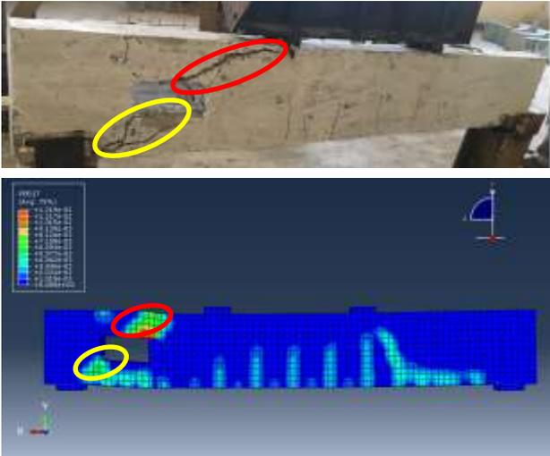
Figure 23 Failure mode for control beam (B2) EXP and FEM.
