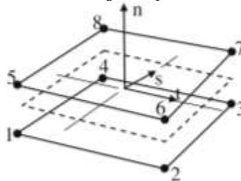
**Figure 15** 8-node 3-D cohesive element.
