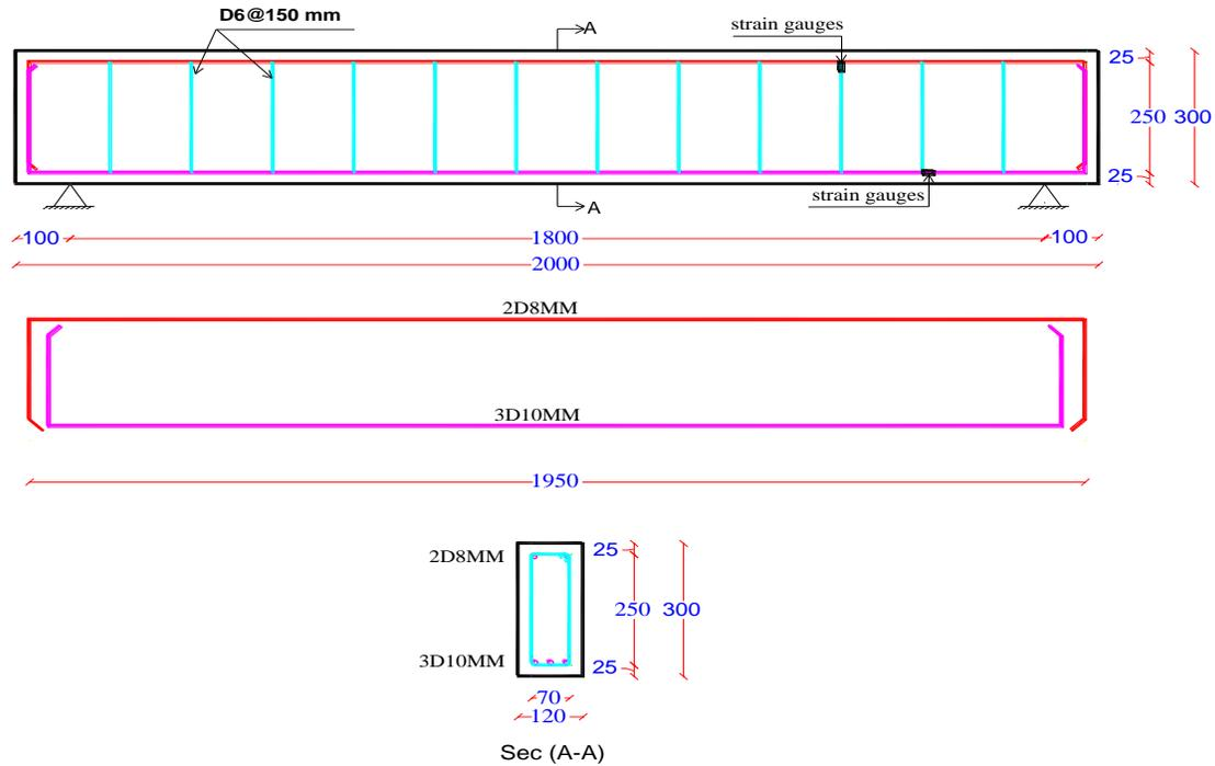
**Figure 2** Detailing of control beam B1 without opening
