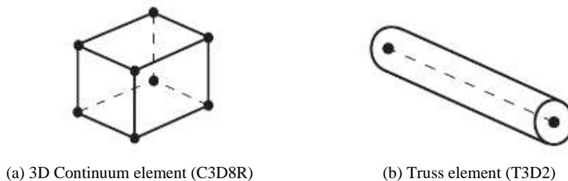
Figure 10 Adopted element models for concrete and reinforcement [15]
