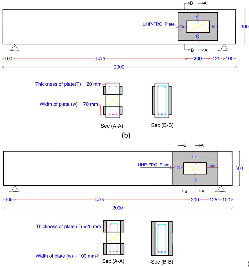
**Figure 5** Geometry and details of strengthened beams (B2) with opening for (Group 3) with different Width UHP-FRC plate specimens.
