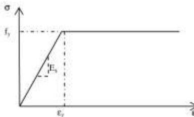
**Figure 13** Stress - strain behaviour of steel.
