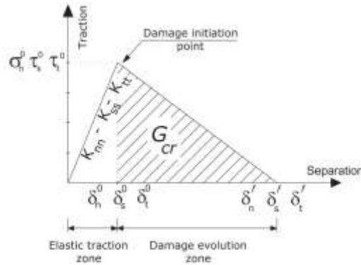
**Figure 14** Description of the traction-separation behavior.
