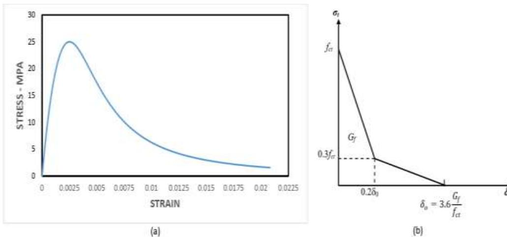
**Figure 11** (a) Stress–strain relationship for concrete under uni-axial compression, (b) tension stiffening model.
