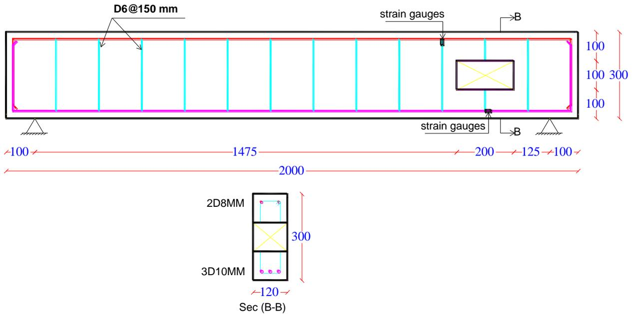
**Figure 3** Geometry of the RC beam (B2) with opening and details of reinforcement.
