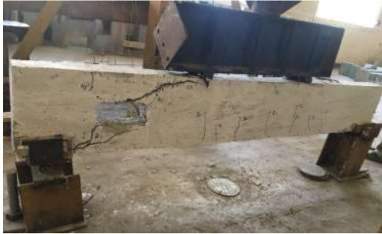
Figure 8 Experimental crack patterns of control beam with openings (B2).
