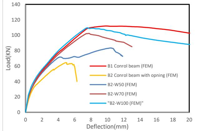
**Figure 21** the load-deflection relationship for the beam B2 with opening strengthening using different width from UHP-FRC plate.
