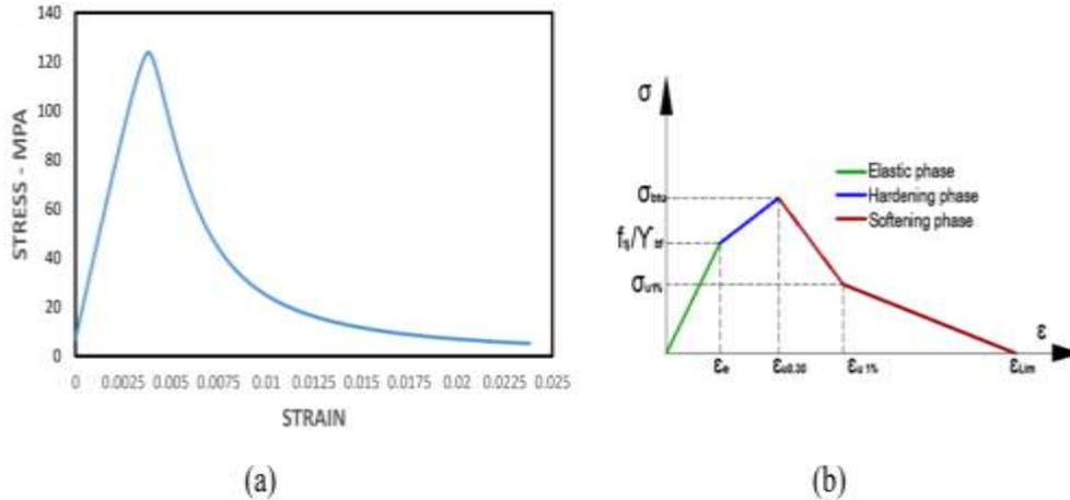
**Figure 12** (a) Stress–strain relationship for UHP-FRC under uni-axial compression, (b) Uniaxial stress- strain curve for UHPFRC [22].
