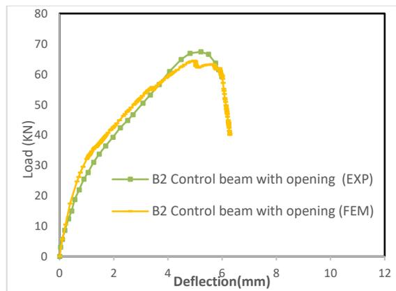
Figure 19 shows the comparison between the experimental and FEM results of the load-deflection relationship for the control beam B2 with opening.
