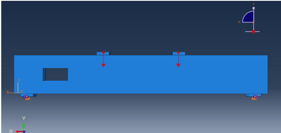
Figure 17 Loading and boundary conditions in ABAQUS.
