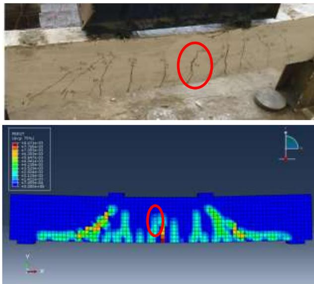
**Figure 22** Failure mode for control beam (B1) EXP and FEM.
