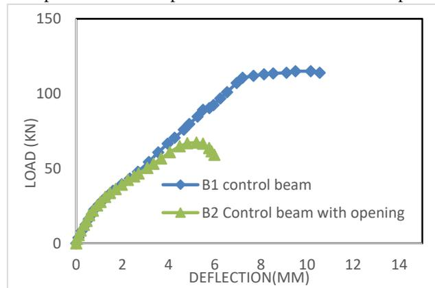
Figure 9 The load-deflection relationship for solid beam (B1) and beam with opening (B2).
