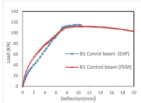
Figure 18 shows the comparison between the experimental and FEM results of the load-deflection relationship for the control beam B1.
