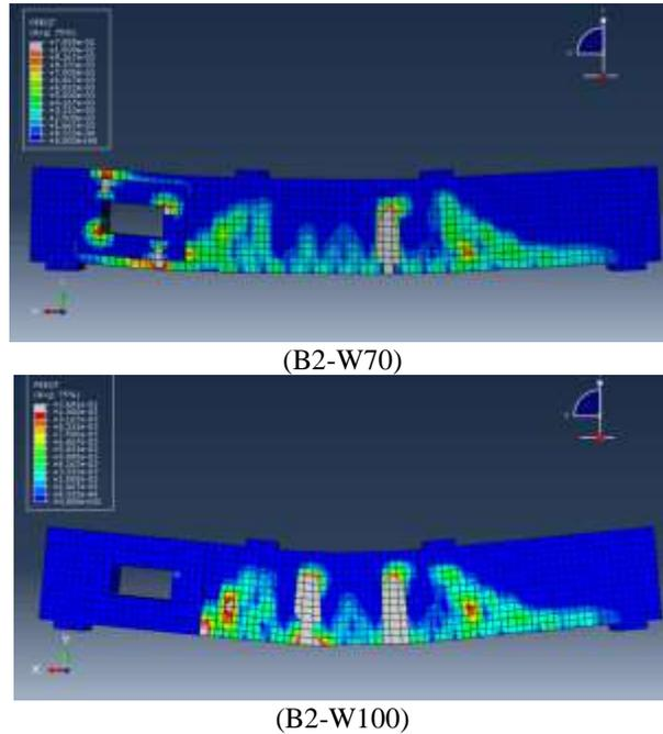
**Figure 25** Failure mode for strengthening beam with opening (B2) with variable width FEM.
