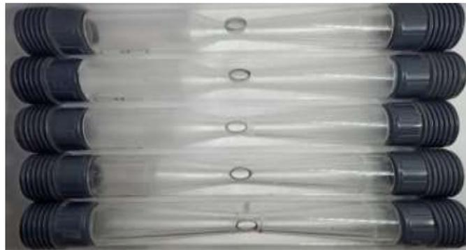
**Figure 5. Photos of the Venturi Tubes (samples).**
