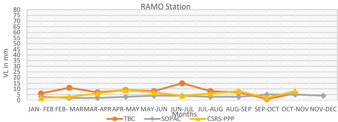
**Figure 3: The Vector Length (VL) for RAMO Station Between Every Two Successive Months by Using Three Techniques in 2018.**
