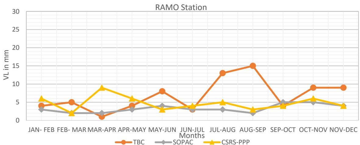
**Figure 7: The Vector Length (VL) for RAMO Station Between Every Two Successive Months by Using Three Techniques in 2019.**
