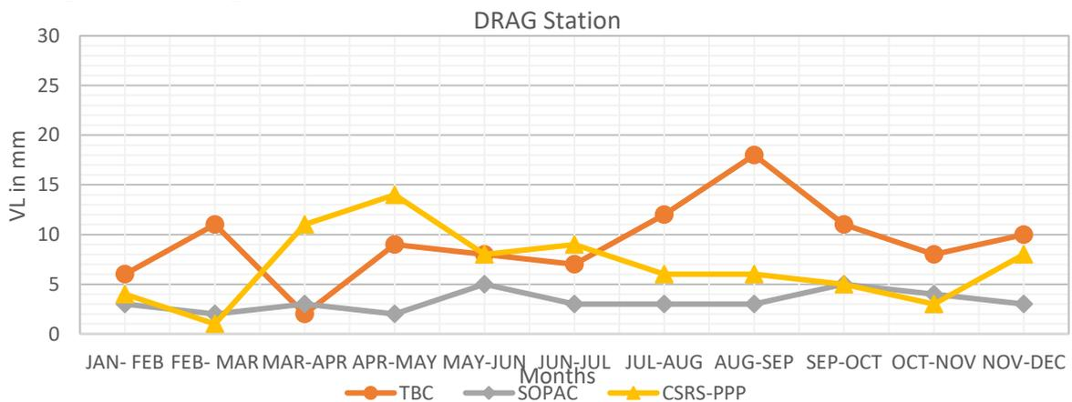
**Figure 6: The Vector Length (VL) for DRAG Station Between Every Two Successive Months by Using Three Techniques in 2019.**
