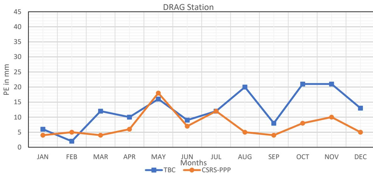
**Figure 14: The Position Error (PE) for DRAG Station Obtained by SOPAC and Other Techniques Monthly in 2019.**
