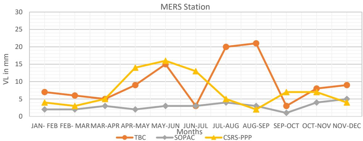
**Figure 9: The Vector Length (VL) for MERS Station Between Every Two Successive Months by Using Three Techniques in 2019.**
