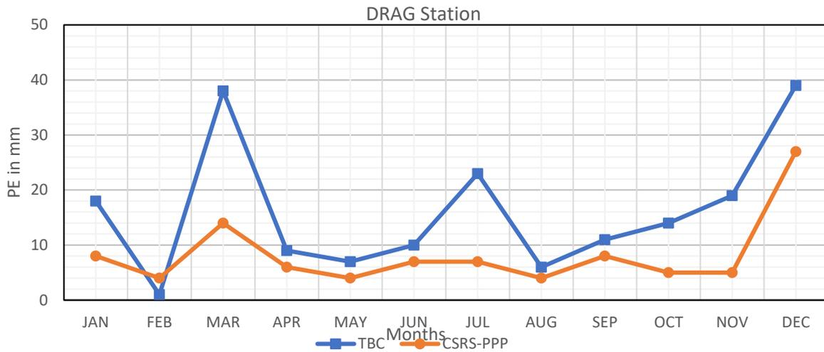
Figure 10: The Position Error (PE) for DRAG Station Obtained by SOPAC and Other Techniques Monthly in 2018.
