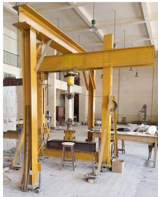
**Fig. 5: General Test Setup**
