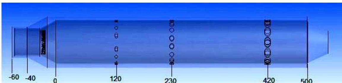
Figure (1) Geometry of the liner of the combustor (All dimensions in millimeters)
