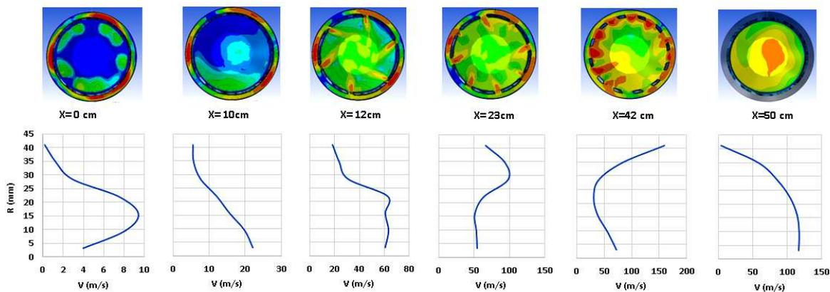
**Figure (4) Radial velocity contour and its distribution at different distance along combustor length.**
