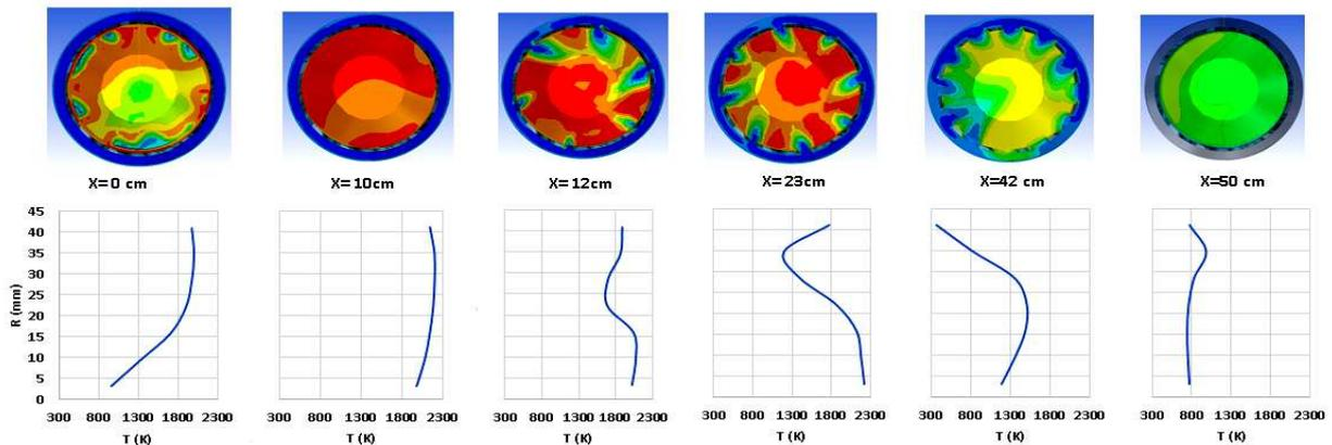
Figure (6) Radial temperature contour and its distribution at different distance along combustor length.
