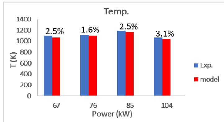
Figure (2) Comparison of the average exit temperature at present model and present experimental
