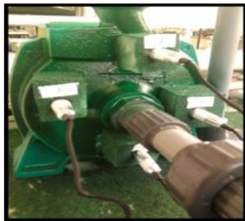
**Fig. 2 Vocal microphones on pump casing**
