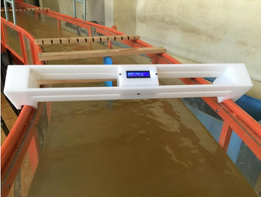
Photo: (2) Measuring device (Ultrasonic device - one spot).
