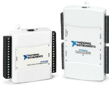
Figure 4: A photograph of the data acquisition NI- 6008 & NI- 6218
