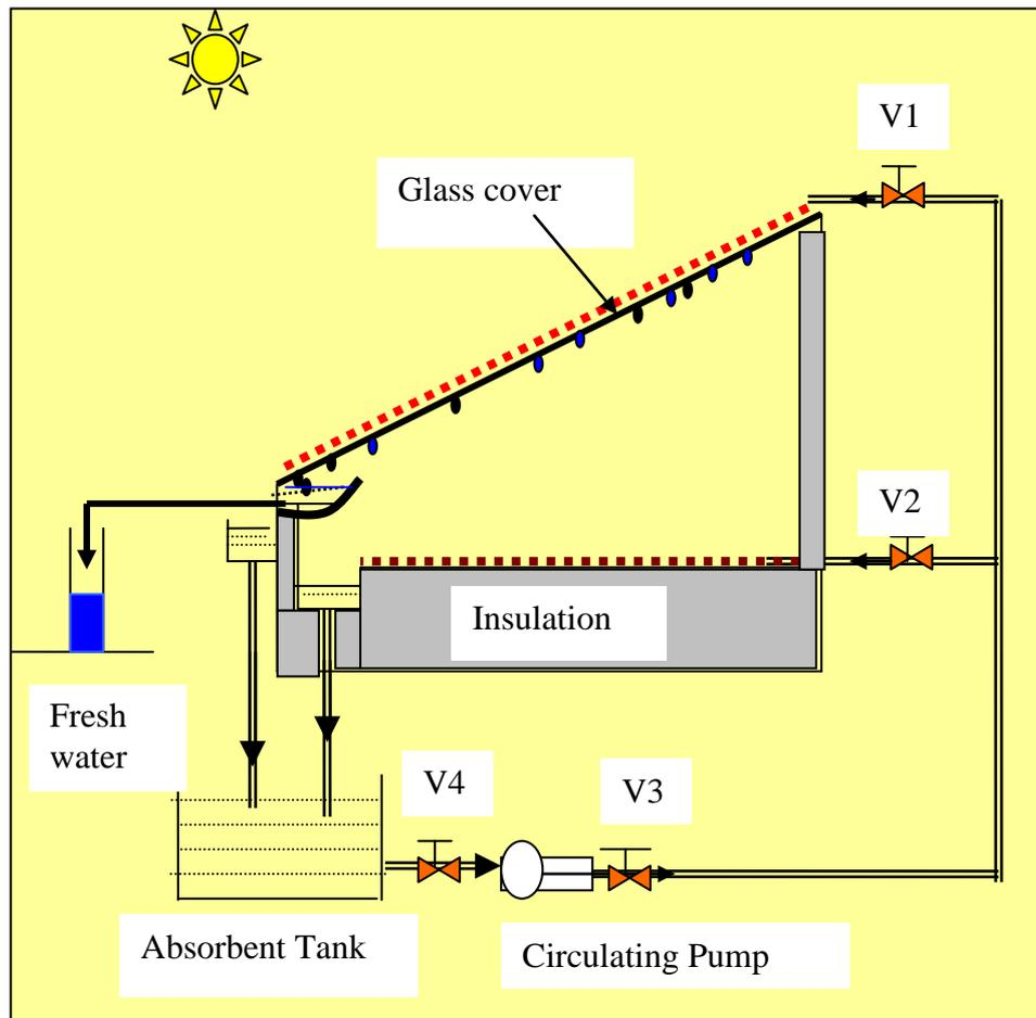
Figure (1) Arrangement unit for water generation from air
