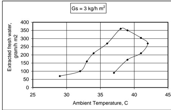
Figure (4) extracted fresh water rate with ambient temperature
