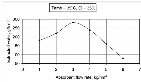
Figure (6) the extracted water rate with absorbent flow rate
