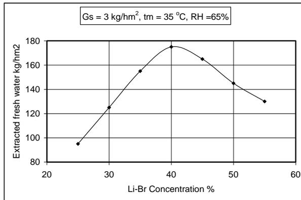
Figure (5) extracted water rate with Lithium Bromide concentration
