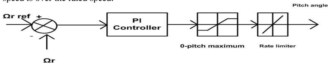
Fig.2. The rotor speed control diagram.
