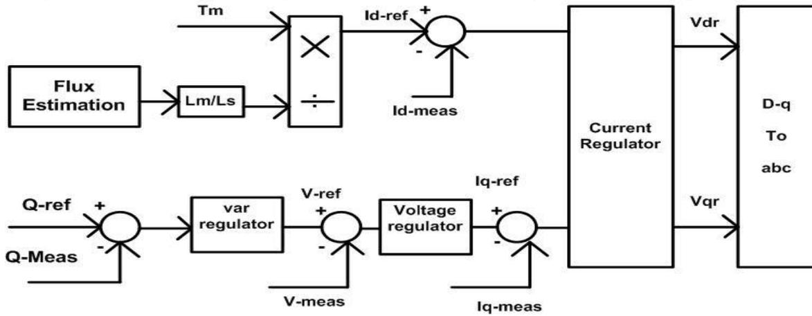
Fig .4. rotor side converter control.
