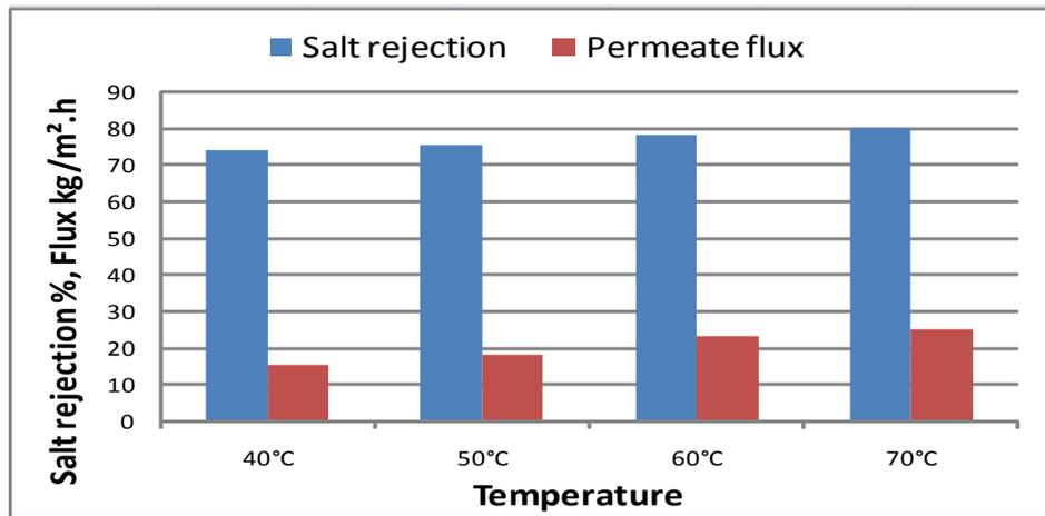
Figure 9: Salt rejection and permeate flux at different temperature values, flow rate, vacuum pressure and salt concentration = 5000 ppm.
