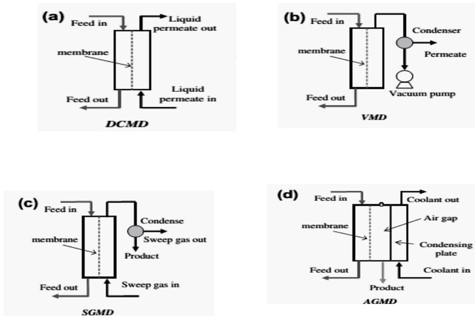
Figure (1) the configurations of the MD (<http://emis.vito.be/techniekfiche>).
