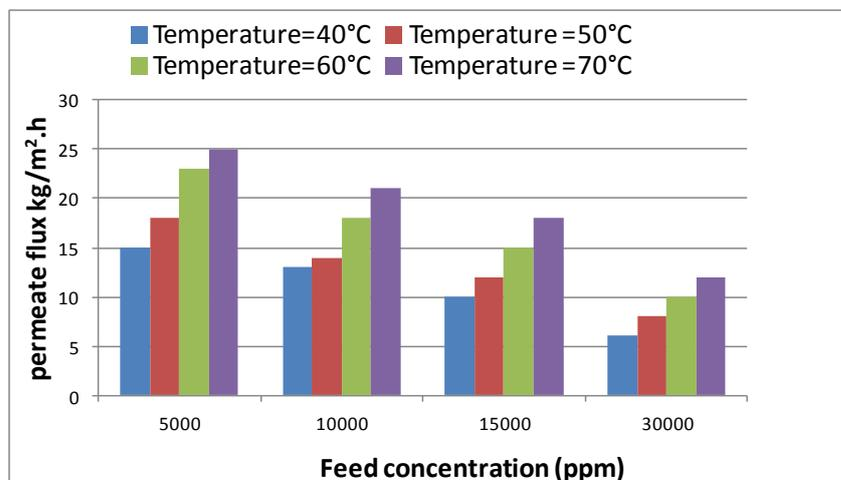
Figure 7 Relation between permeates flux and feed concentration at different temperature values, Constant flow rate = 1 L/min, and constant vacuum pressure = 0.4 bar.
