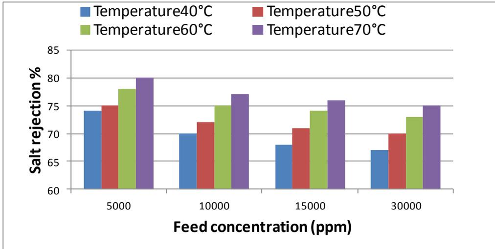
Figure 8: Salt rejection and feed concentration at different temperature values, flow rate = 1 L/min, and vacuum pressure = 0.4 bar
