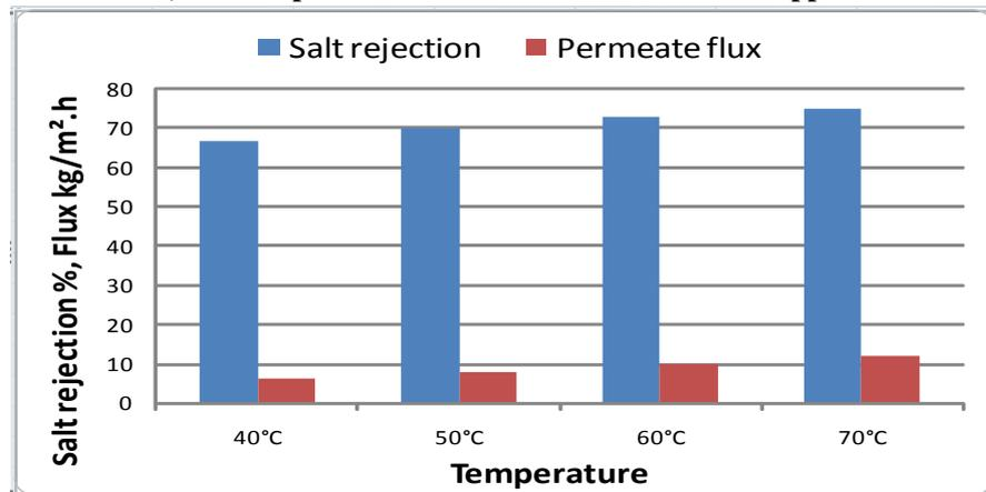
Figure 10: Salt rejection and permeate flux at different temperature values, Flow rate, vacuum pressure and salt concentration = 30000 ppm.
