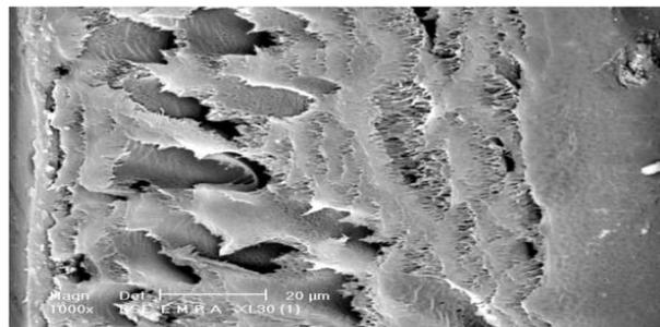
Figure (3) Crosssection of the Membrane
