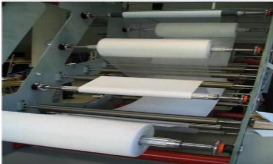
Figure (2) (A) Flat sheet membrane.
