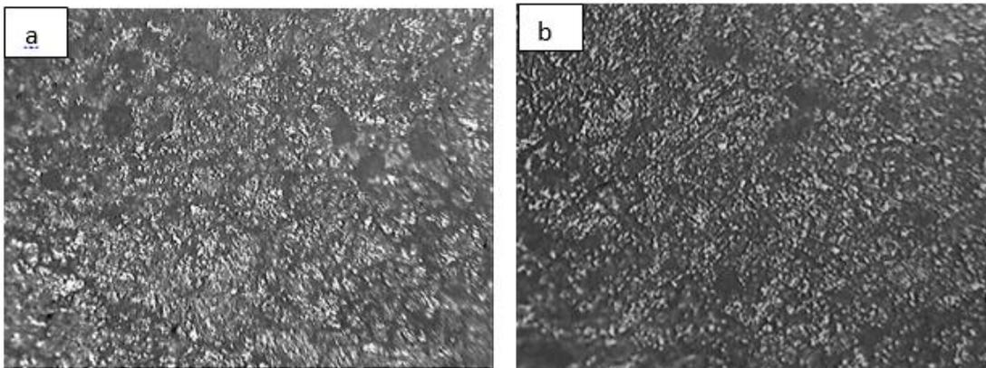
Fig.4: Optical micrographs of composites reinforced with A356 alloy+ 20%: (a) As cast, (b) Heat treated (100 X)
