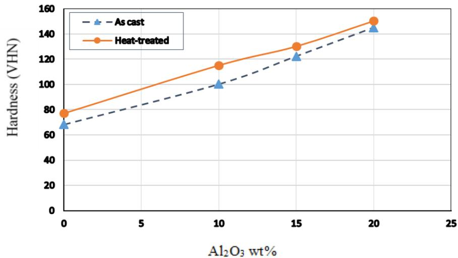
Fig.3: Effect of heat treatment on hardness of the test specimens
