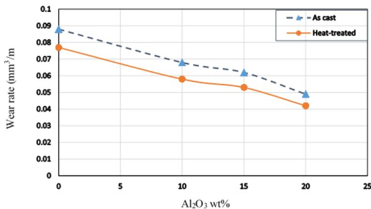
**Fig.5: Effect of heat treatment on wear rate of the test specimens**
