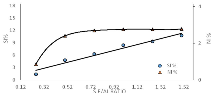
Figure 3 Effect of  $\text{Na}_2\text{SiF}_6/\text{Al}_{\text{total}}$  wt. ratio on the Si% and Ni% of the prepared Al-Si-Ni ternary alloys.
