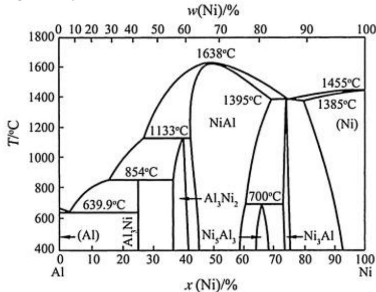
Figure 7 Al-Ni binary phase diagram [16]
