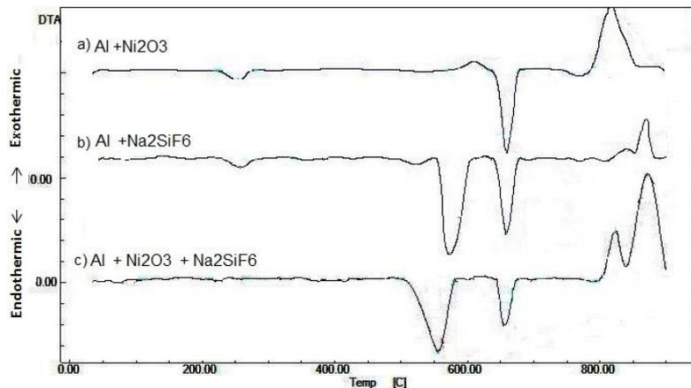
Figure 2 Differential thermal analysis (DTA) a)  $\text{Ni}_2\text{O}_3 + \text{Al}$ , b)  $\text{Al} - \text{Na}_2\text{SiF}_6$  and c)  $\text{Al} + \text{Na}_2\text{SiF}_6 + \text{Ni}_2\text{O}_3$  mixtures
