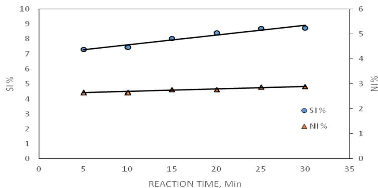
Figure 5 Effect of reaction time on the Si% and Ni% of the prepared Al-Si-Ni ternary alloys
