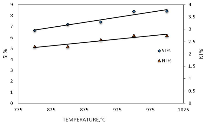
Figure 1 Effect of temperature on the Si% and Ni% of the prepared Al-Si-Ni ternary alloys
