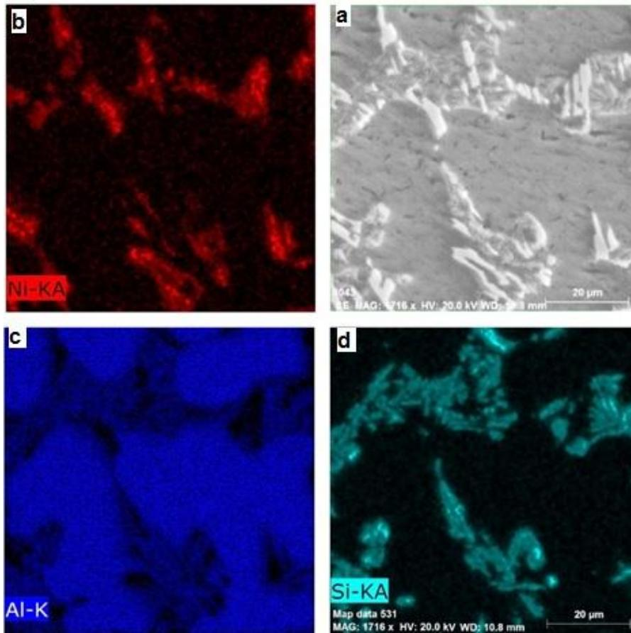
Figure 9 EDX mapping of hypoeutectic Al-Si-Ni ternary alloy containing 8.4 Si and 2.75 Ni.
