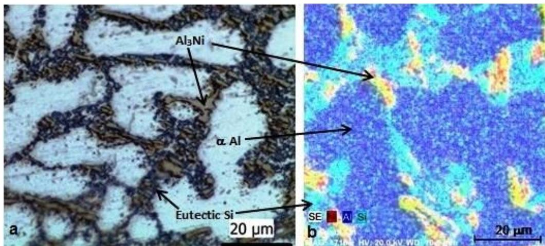
Figure 8 (a) LOM and (b) SEM images of hypoeutectic Al-Si-Ni alloy containing 8.4 Si and 2.75 Ni, etched by 0.5% HF acid.
