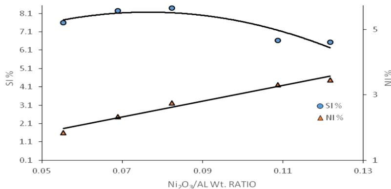
Figure 4 Effect of  $\text{Ni}_2\text{O}_3 / \text{Al}_{\text{total}}$  wt. ratio on the Si% and Ni% of the prepared Al-Si-Ni ternary alloys
