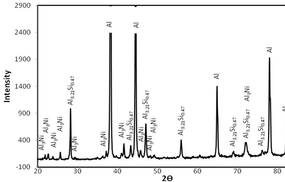
Figure 6 XRD diffraction for the produced Al-Si-Ni ternary alloy containing 8.4 Si and 2.75 Ni.
