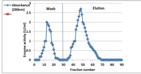
Fig.1: Ion exchange chromatography on DEAE cellulose column (3x 20cm).
