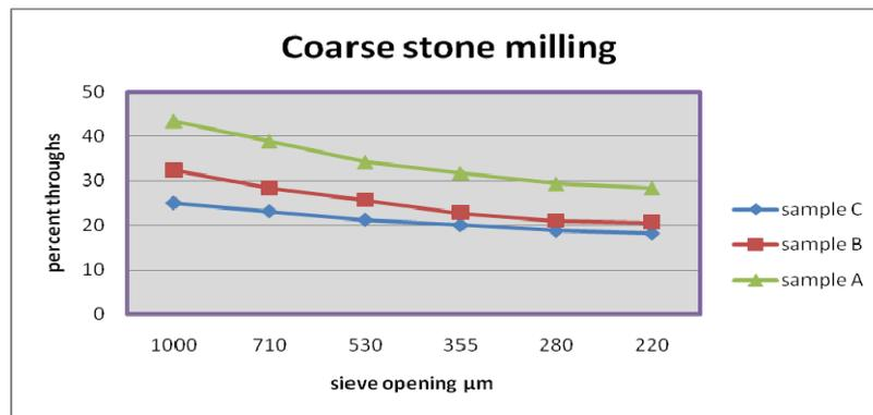
Fig. 3: Coarse stone mill flour granulation curve
