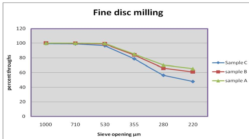
Fig. 2: Fine disc mill flour granulation curve
