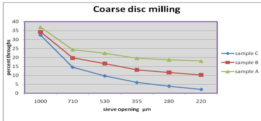
Fig. 4: Coarse disc mill flour granulation curve
