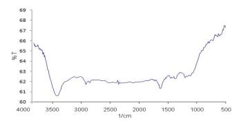
Fig. 4: FTIR spectrum recorded by making KBr disc with synthesized gold nanoparticles synthesized.
