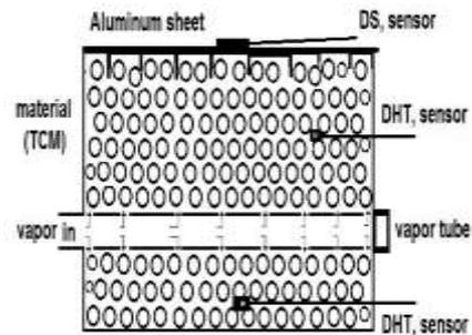
**Fig 3.** The storage material container covered with aluminum sheets and sensors locations, where: - DS measures aluminum sheet surface temperature, DHT sensor measures storage material temperature
