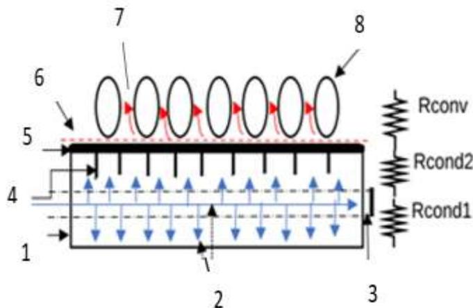
**Fig 7.** Illustration of the process of recovering thermal process and heat transfer from TCM to the aluminum sheet to eggs where: - 1- the storage material container, 2- vapor flow, 3- perforated vapor pipes, 4- fins, 5- aluminum sheet, 6- the egg tray, 7- heat flow, 8- egg
