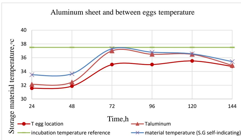
**Fig 15.** The average temperature for aluminum sheet and eggs location with storage material Silica gel self-indicating
