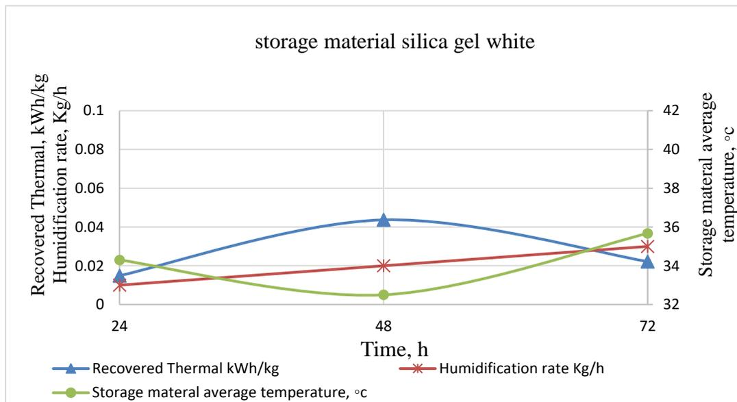
Fig 10. The recovered thermal and temperature of storage material with humidification rate of storage material (commercial white Silica gel)
