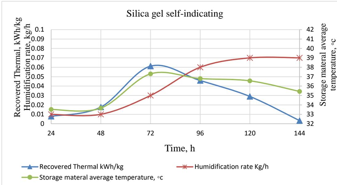
Fig 9. The recovered thermal and temperature of storage material with humidification rate of storage material (Silica gel self-indicating)
