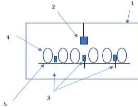
**Fig 6.** sensors location inside traditional poultry egg incubator, 1-incubator body, 2- DHT22 - temperature & humidity sensors, 3- DS 18B20 – temperature sensors, 4- egg, 5- egg tray
