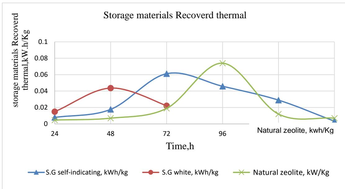
**Fig 8.** Illustrate the recovered thermal, in (kW.h/kg) of storage materials (Silica gel self-indicating, Silica gel white, and Natural Zeolite) during the time
