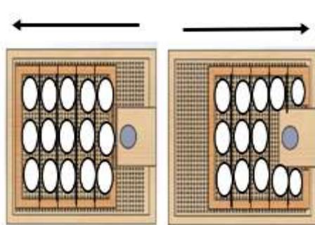
**Fig 2.** The egg tray with 25 eggs and turning motor capacity, the eggs turn straight forward and back.
