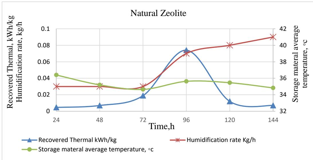
Fig 11. The recovered thermal and temperature of storage material with the humidification rate of storage material (Natural Zeolite)
