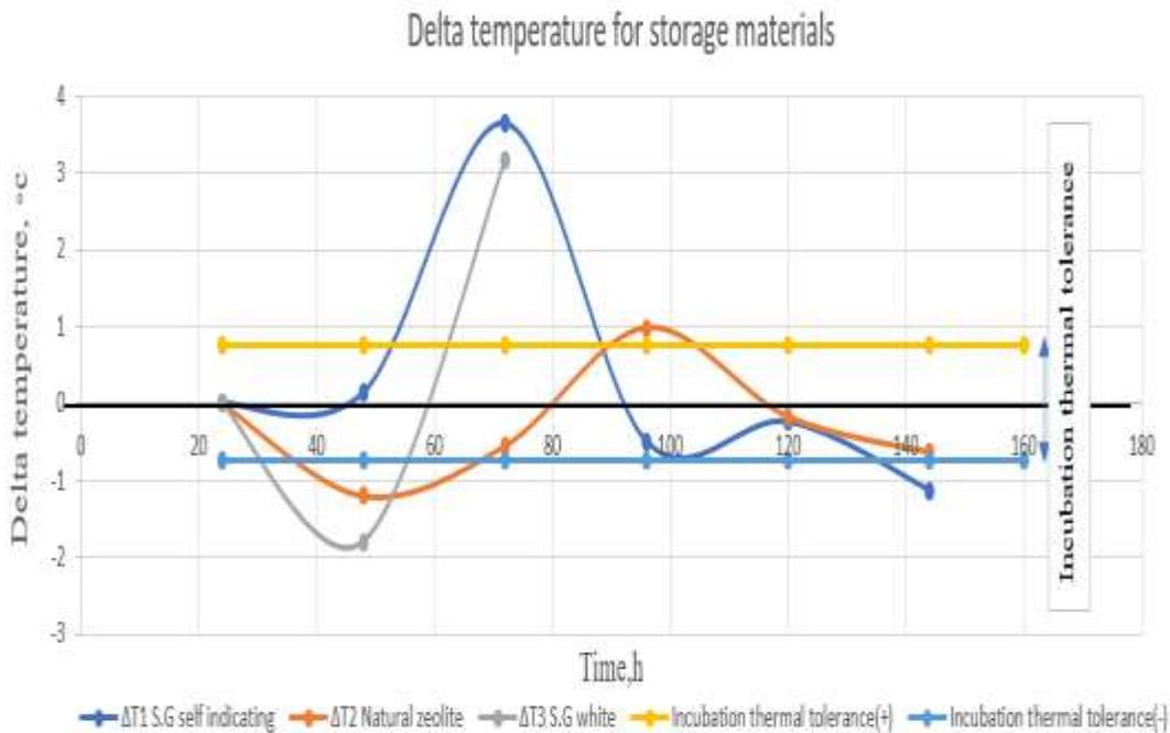
Fig 12. Delta temperature for storage material (Silica gel self-indicating, white Silica gel and Natural Zeolite) and incubation thermal tolerance for chicken eggs
