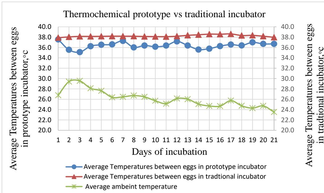
Fig 16. The average of temperature between eggs in thermochemical prototype and traditional incubator
