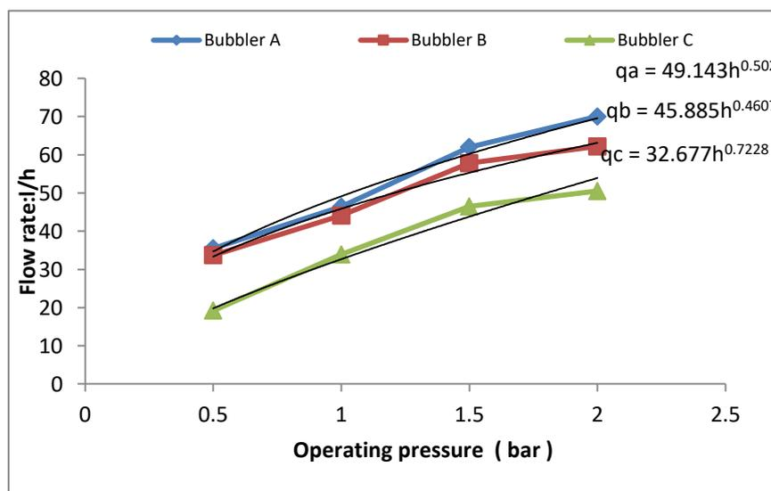
Fig. 2. Calibration of bubbler
