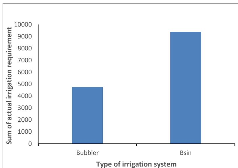
**Fig. 3.** Comparison between the actual irrigation requirement of date palm under basin & bubbler irrigation system
