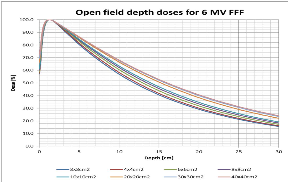
**Fig. (4): Percentage Depths Dose for All field size start from 3cm<sup>2</sup> to 40cm<sup>2</sup> for 6 MV (FFF)**
