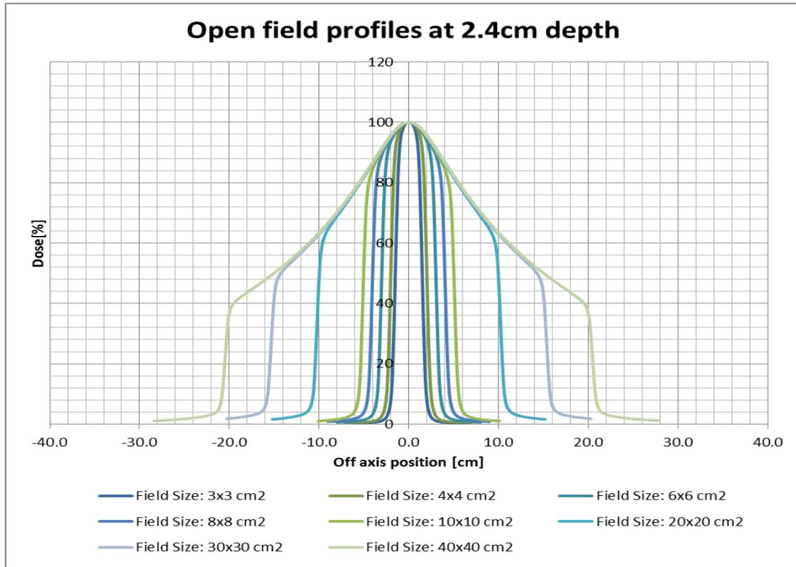
**Fig. (7): Beam profiles for all field size start from 3cm<sup>2</sup> to 40 cm<sup>2</sup> for 10 MV (FFF) at depth 24.0 mm**
