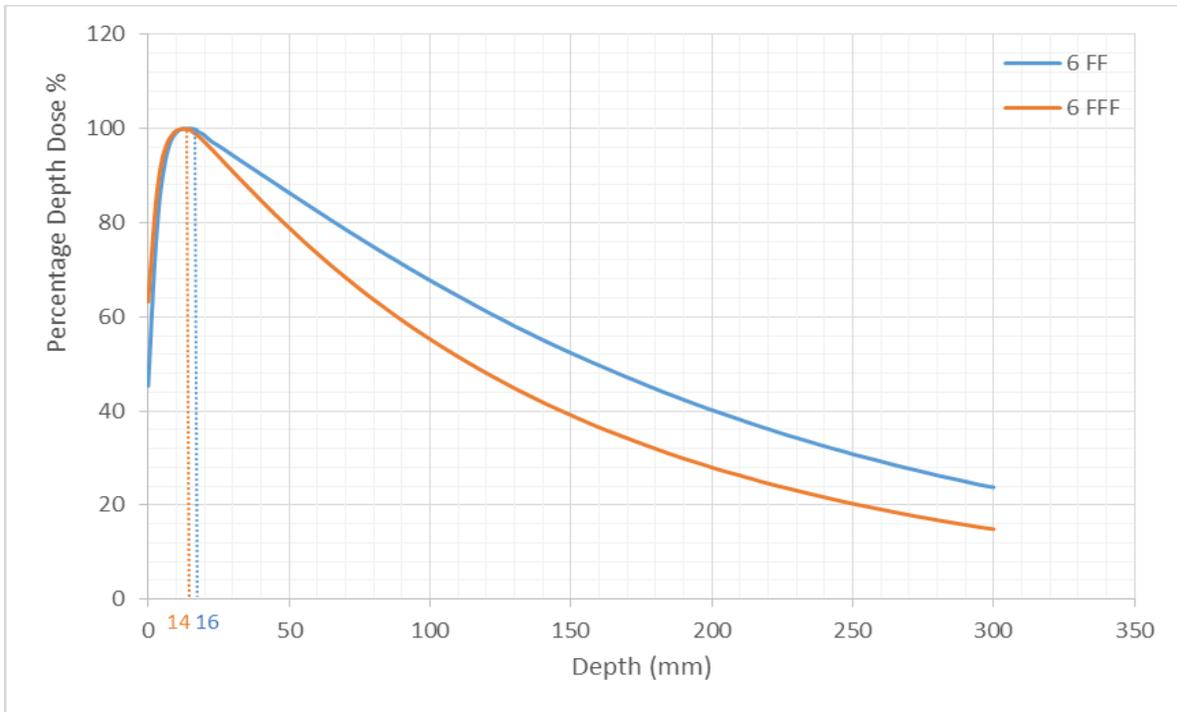
**Fig. (5) Comparison between PDD% Curve of (6FF& 6FFF) at Field size 10 x 10 cm<sup>2</sup> and at SSD 100 cm.**
