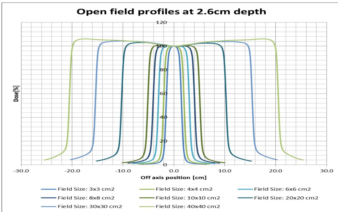
**Fig. (6): Beam Profiles for All field size start from 3cm<sup>2</sup> to 40 cm<sup>2</sup> for 10 MV (FF) at depth 26.0 mm.**
