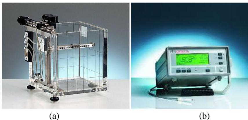
**Fig. (2): MP3 water phantom (a) and PTW-UNIIDOS electrometer (b).**
