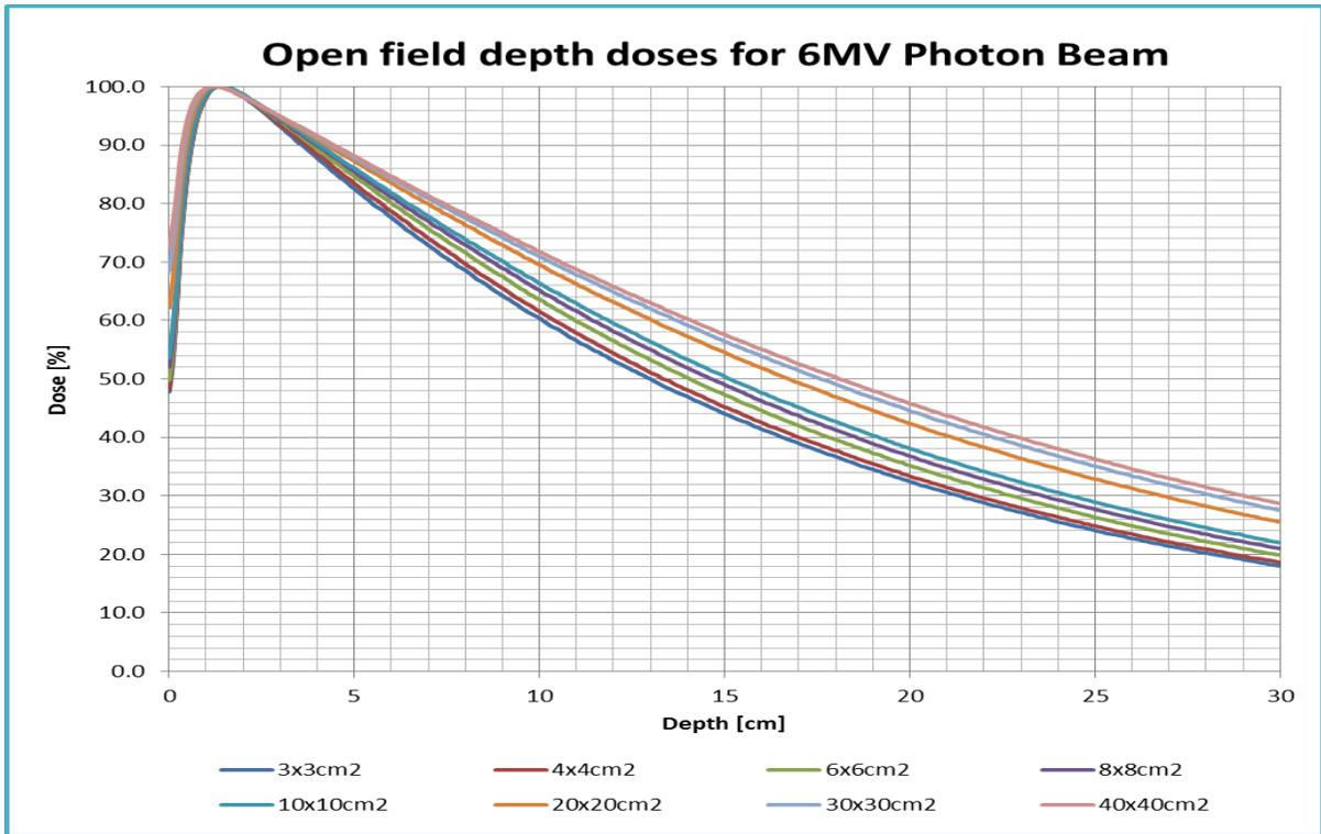
**Fig. (3): Percentage Depths Dose for all field size start from 3cm<sup>2</sup> to 40cm<sup>2</sup> for 6 MV (FF).**
