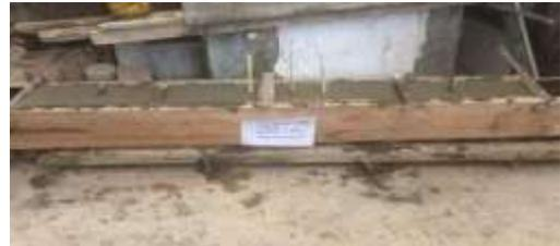
Fig. 3. Casting of Beams
