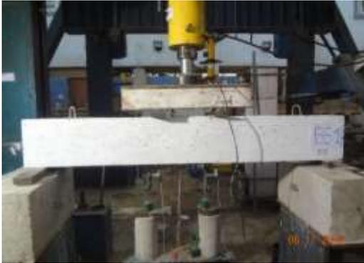
Fig. 7. Test setup for four-point bending Test of Beam
