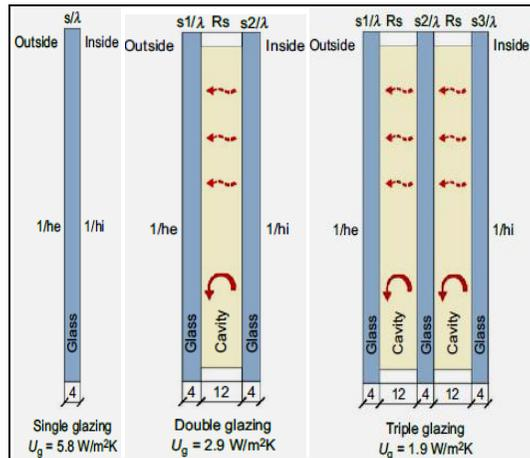
Fig. (1): Thermal transmittance of a single-glazed, double-glazed, and triple-glazed window<sup>(8)</sup>.
