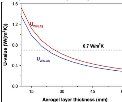
Fig. (8): Influence of thickness and particle size (Aerogel-AS: small granules, blue line; Aerogel-AB: Large granules, red line) of aerogel on thermal performance <sup>(1)</sup>
