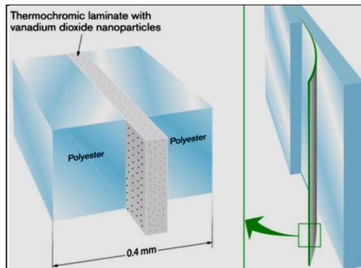
Fig.5: Conceptual sketch of a thermochromic foil incorporating a laminate with VO<sub>2</sub>-based nanoparticles between two foils of (polyester, PET) <sup>(1)</sup>
