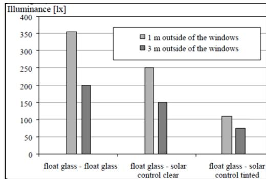
Fig. (3): Comparison of internal luminance on the working plane in the reference room with different window glazing <sup>(11)</sup>
