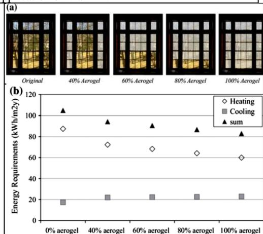
Fig. 14 The investigated window configurations with different percentages of aerogel inclusion (a); heating and cooling energy requirements for different window systems (b) <sup>(1)</sup>
