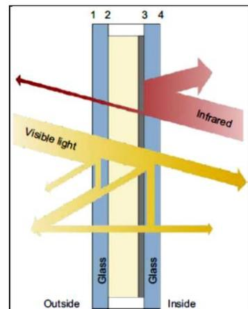
Fig. (2): Double glazing with Low-e coating<sup>(8)</sup>.
