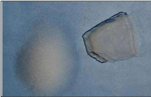
Fig. (7): Silica aerogels: granular (left) and monolithic pane (right) <sup>(1)</sup>
