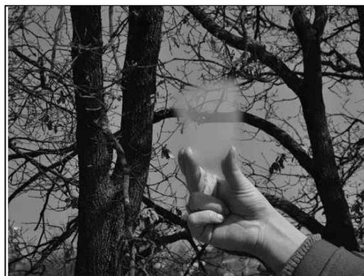
Fig.(6) View through a monolithic aerogel sample <sup>(5)</sup>
