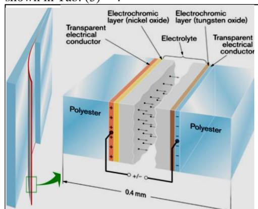
Fig. (4): Construction principle for an electrochromic foil device. The entire foil can be used as a laminate between two glass panes <sup>(1)</sup>.
