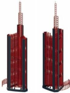
Fig 43 : The two composite mega columns
