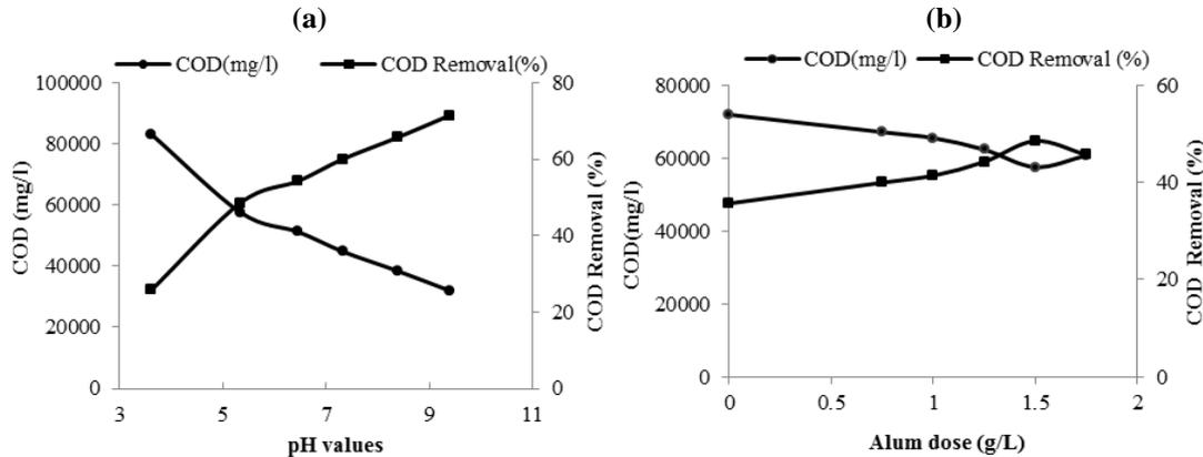
Figure (2): Coagulation/Precipitation process using alum (a) Determination of optimum dose of alum, (b) Determination of optimum pH at 1.5g/L alum dose.
