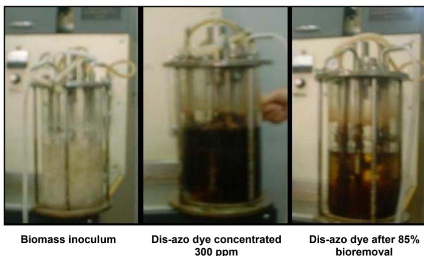
**Figure (1a):** Decolorization of direct brown dye by *A. niger* strain at  $\frac{1}{2}$  v/v/min aeration rate after 24 hrs incubation.
