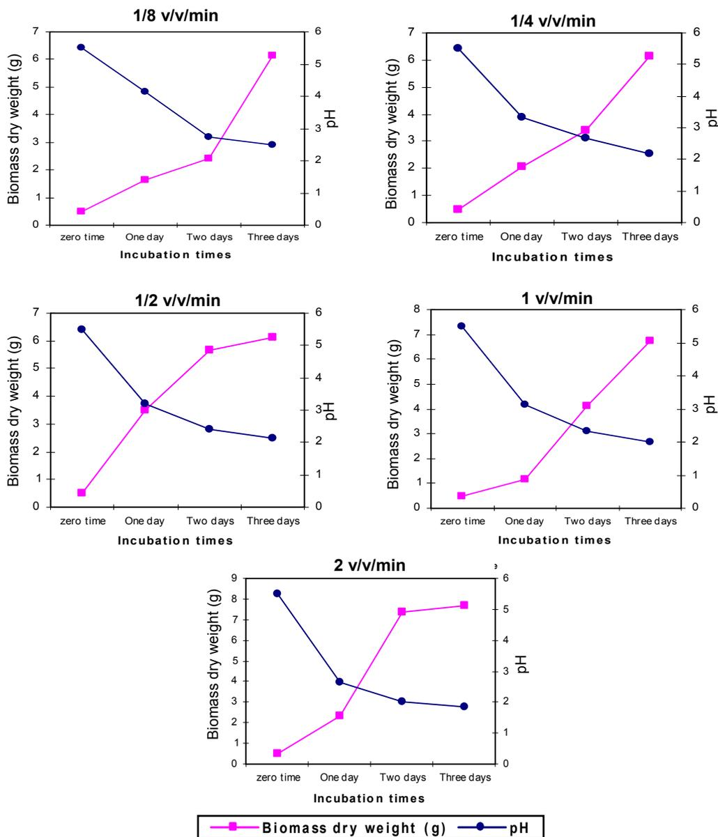
**Figure (5):** Effect of aeration on accumulation of fungal biomass and pH changes on sucrose-yeast medium.
