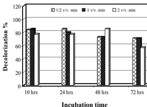
**Figure (2):** Effect of aeration on removing of dis-azo dye using fungal strain 20 (after addition 300 ppm dye (10, 24 hrs), and another 600 ppm (48, 72 hrs).
