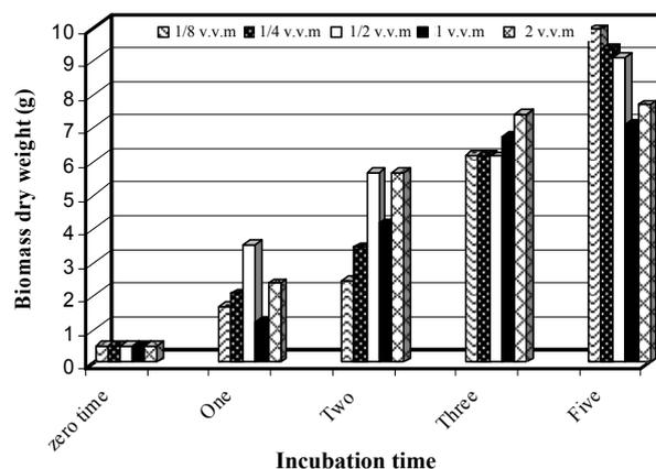
**Figure (3):** Effect of aeration on accumulation of fungal biomass grown on sucrose-yeast medium.
