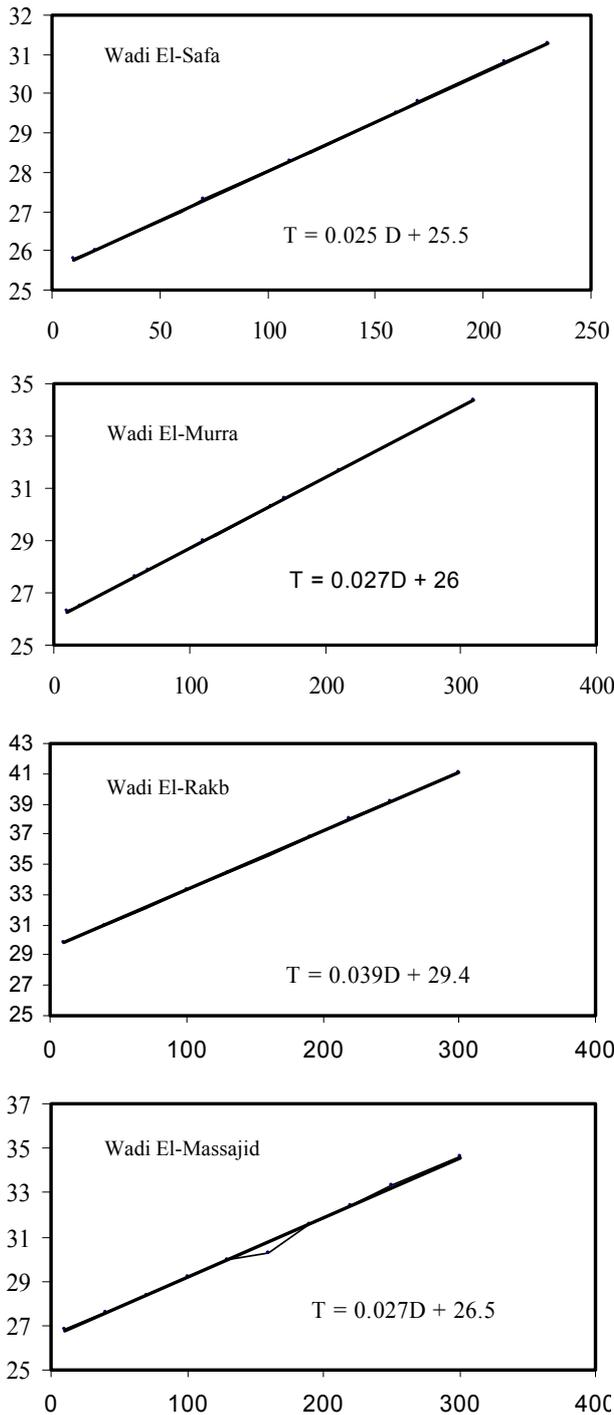
**Figure (5):** The relations between depth (m) and temperature (°C) of the study area.
