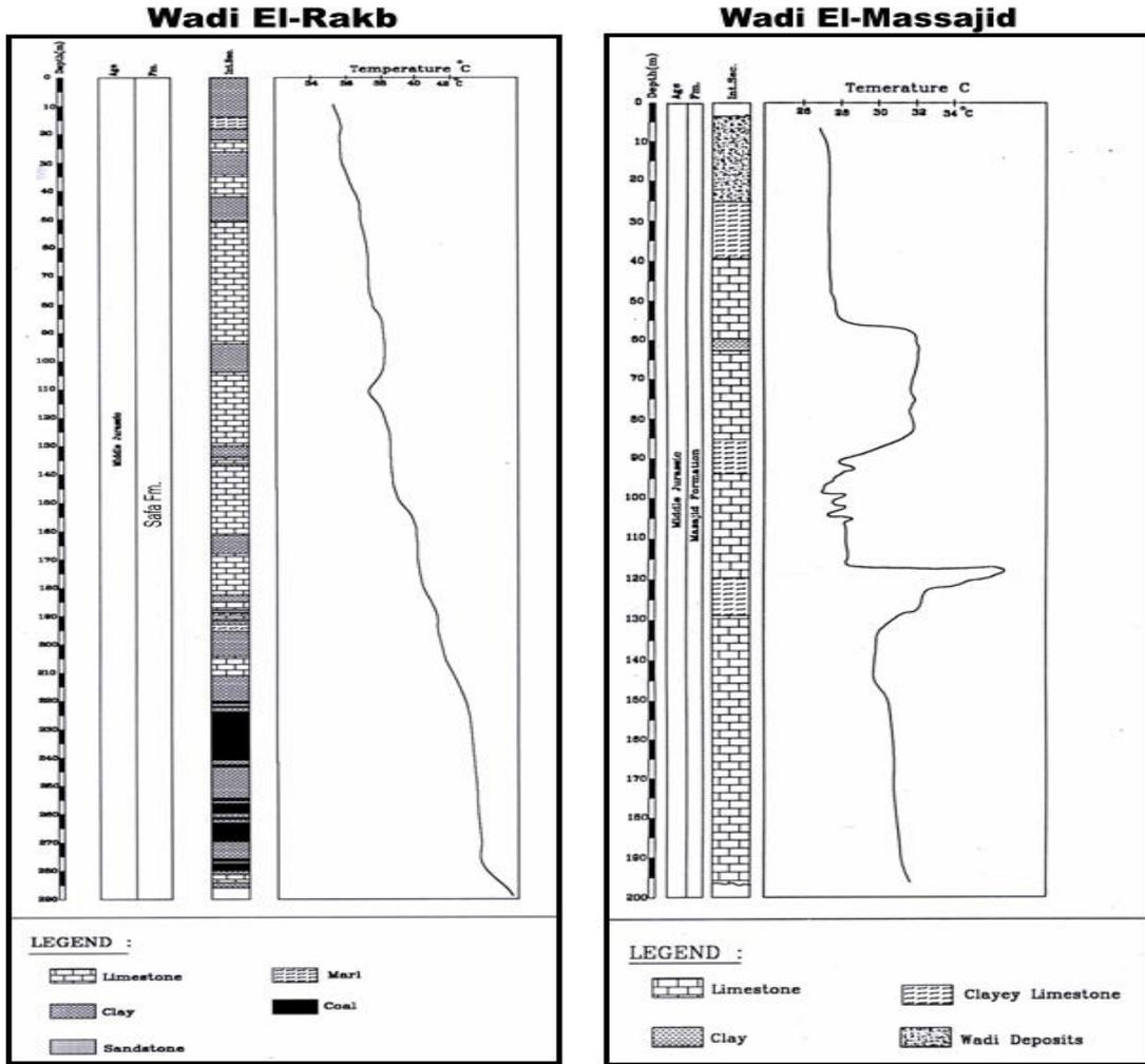
Figure (6): Temperature – Depth Curves at Wadi El-Rakb B.H.No.8 and Wadi El-Massajid B.H.No. 2
