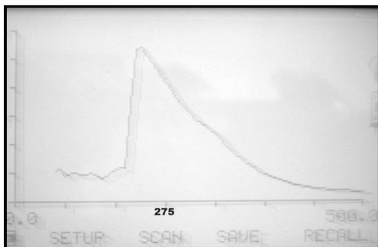
**Figure (4):** Formation of aromatic amines as a result of dye biodegradation (Aromatic amine peak at UV spectrophotometer at 275nm).
