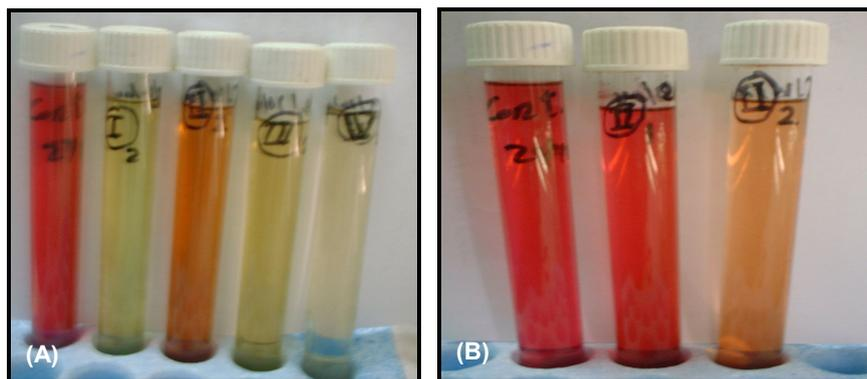
**Figure (1): (A and B)** Removal of Remazol red dye using enrichment cultures of four wastewater samples under aerobic and anaerobic conditions.
