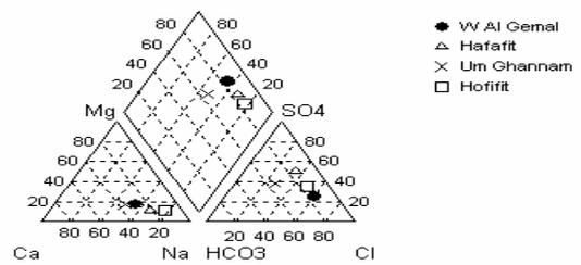
**Figure (5):** Trilinear Piper diagram of water chemistry in the study area.
