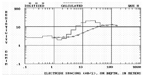
**Figure (5):** Example of an interpreted VES curve for VES No. 8 according to Zohdy and Bisdorf method (1989).
