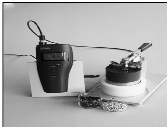
Figure (1): Portable hygrometer (Digital Humidity Sensors). The Rotronic Palm 3 display unit with AWVC-dio workstation utilises a dry state hygrolytic sensor and in-built fan for rapid equilibration. Range: +5 to +50 °C (+/- 0.2°C), 0 to 100% RH (+/- 1.5% RH)
