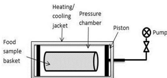
**Fig. 1. Diagram showing components of high pressure system.**
