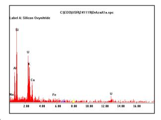
Fig. (3): The scan of the original sample which shows the existence of uranium with iron, aluminium, alkali metals and silicon.
