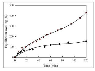
Fig. (4): Time dependent swelling of equi-weight MAAc/ PEOz at  $(\bullet)$  pH 1 and  $(\triangledown)$  pH 7.
