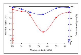
Fig. (1): Effect of the aqueous feed solution composition on the ( $\blacksquare$ ) conversion and ( $\bullet$ ) gelation degree of PEOz/MAAc copolymer. Irradiation dose: 15 kGy and Feed solution concentration 15 wt%.
