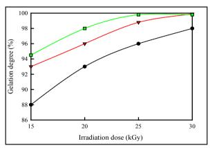
Fig. (2): Effect of the Irradiation dose on the gelation degree of PEOz/AAc copolymer at different feed solution concentration; (●)15, (♥)20 and (■)25 wt%. Aqueous feed solution composition(MAAc/PEOz): (50:50 wt%).
