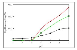
Fig. (3): pH-dependent swelling of MAAc/PEOz copolymer hydrogels of different MAAc content; (•) 35, (•) 50 and ( $\mathbf{\nabla}$ ) 90 wt%. Feed solution concentration 20 wt%, irradiation dose 20 kGy.
