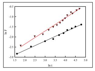
Fig. (5): Linear dependence of  $\ln F$  on  $\ln t$  of equi-weight MAAc/PEOz at (•) pH 1 and ( $\mathbf{\nabla}$ ) pH 7.
