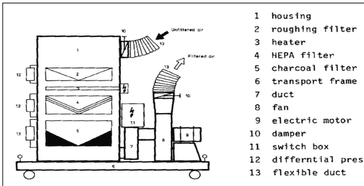
Fig. (4): A Modular and Mobile Filter Units Schematic.
