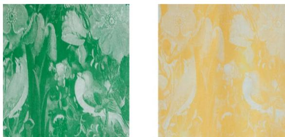
Figure 5: Thermochromic colorant effect
