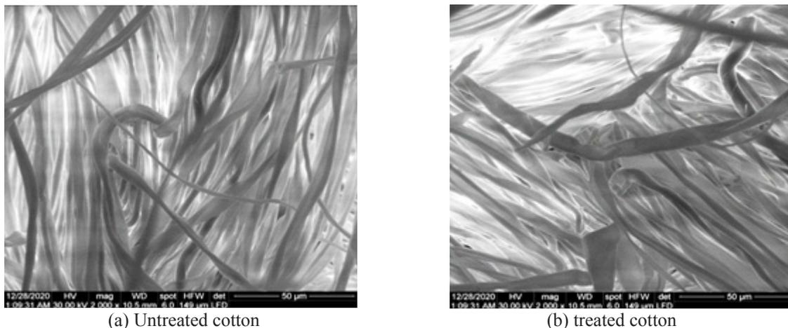
**Fig. 3. SEM images of untreated and treated cotton fabrics with ZnO nanoparticles**
