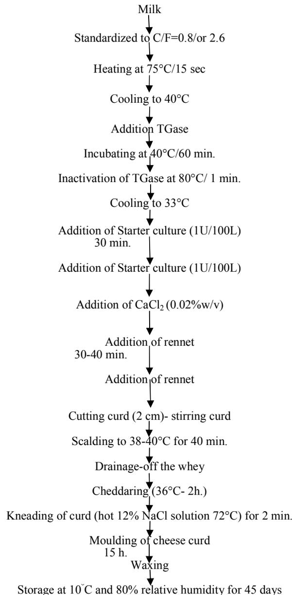
**Fig (1):** Flow sheet of the production of Kashkaval cheese treated with TGase
